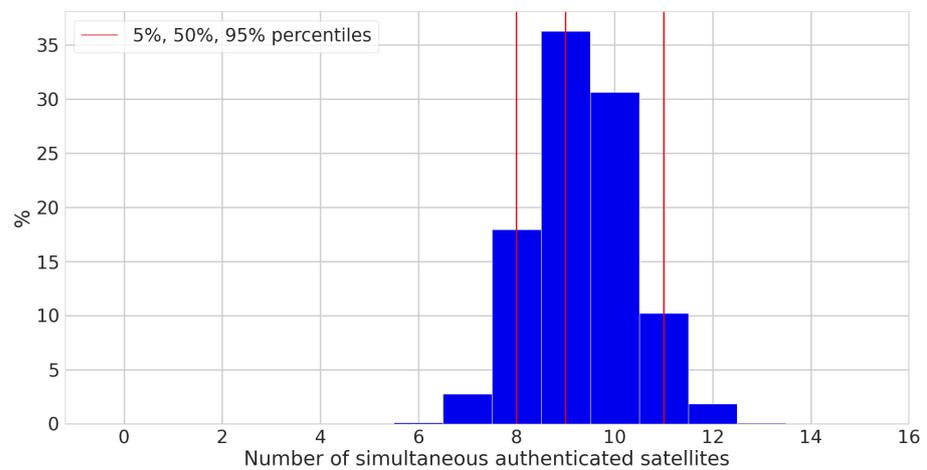
**Figure 4.** Distribution of the number of simultaneously authenticated satellites available during our tests.
