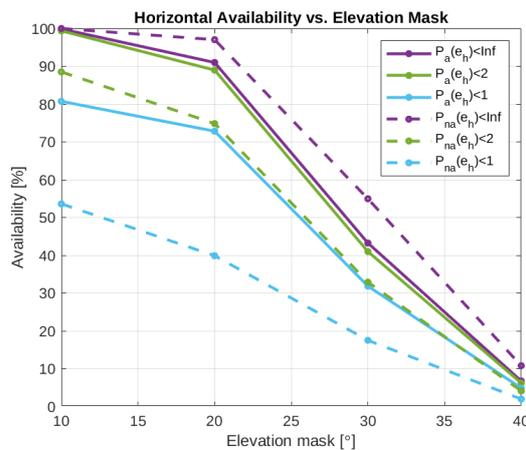
Figure 11. Horizontal availability versus the elevation mask. The colors indicate different error thresholds for the availability. The solid line corresponds to the authenticated positioning solution availability and the dashed line corresponds to the regular non-authenticated positioning solution availability.
