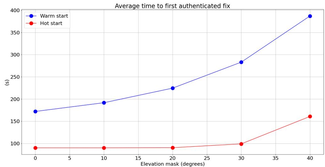
**Figure 6.** Average TTFAF as a function of the elevation mask.
