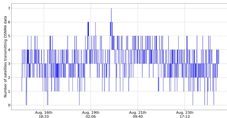
**Figure 8.** Number of satellites above 30 degree elevation transmitting OSNMA data during August 2023.
