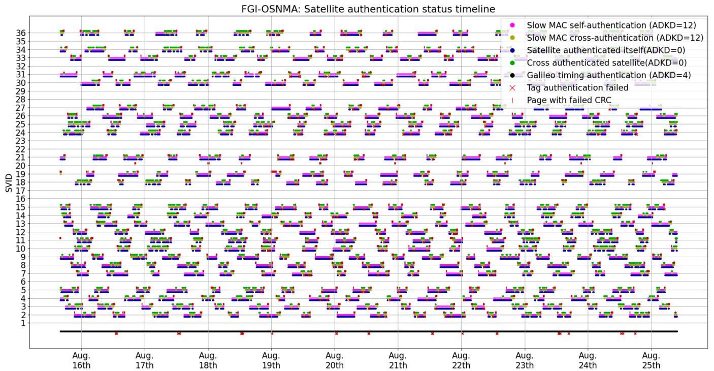
**Figure 1.** Authentication events over the test period. Note that the red markers slightly below the line are tag authentication failures, while the red markers slightly above the line are CRC failures.
