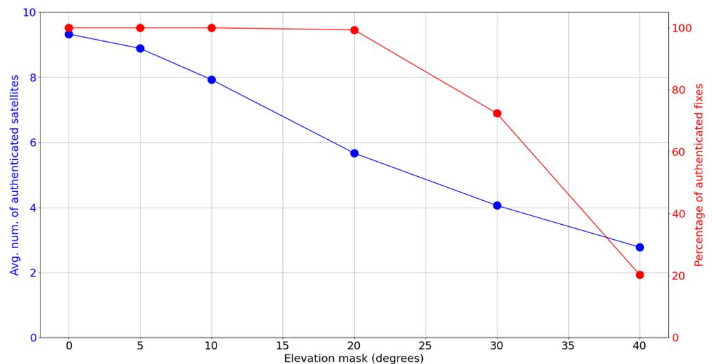
**Figure 5.** Average number of satellites with authenticated status (blue) and percentage of authenticated fixes (red) as a function of the elevation mask.
