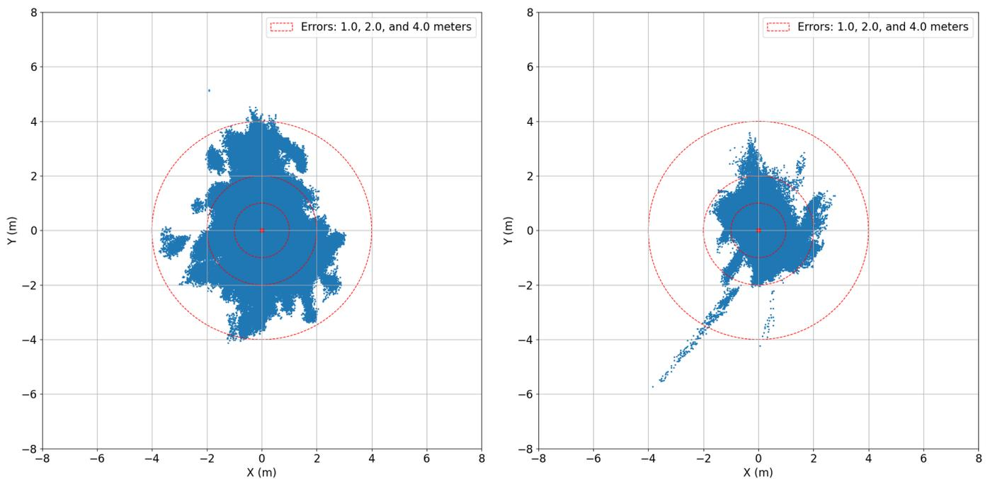
**Figure 9.** Unauthenticated positioning (**left**). Authenticated positioning (**right**) with no OSNMA processing elevation mask. Both use a 10 degree elevation mask in positioning. The availabilities of the positioning solutions can be found in Table 5.
