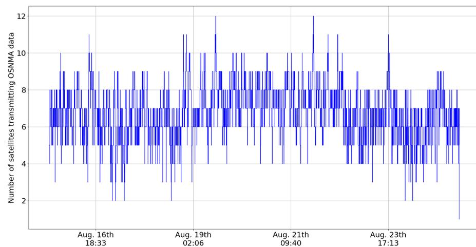
**Figure 7.** Number of satellites transmitting OSNMA data during August 2023.
