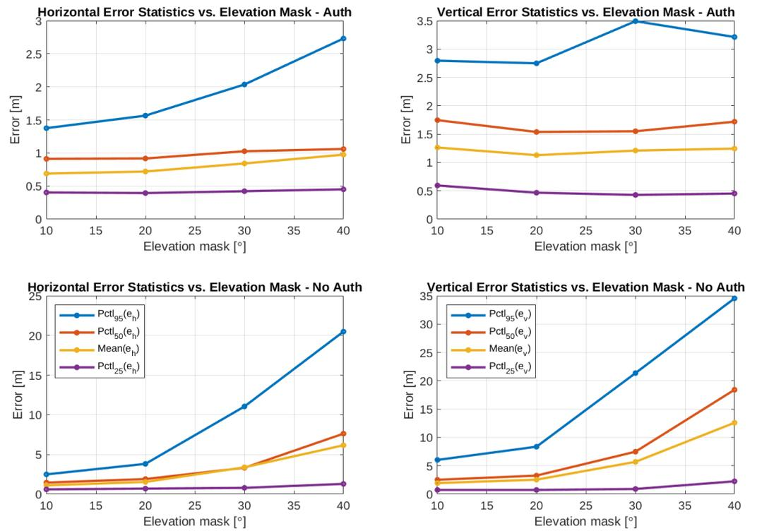
Figure 10. Positioning error mean and percentiles versus the elevation mask.
