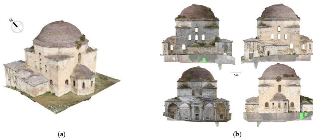
**Figure 24.** Products of the TLS–photogrammetric data fusion: (a) textured 3D model; (b) facade orthophotos (east, west, north, south).
