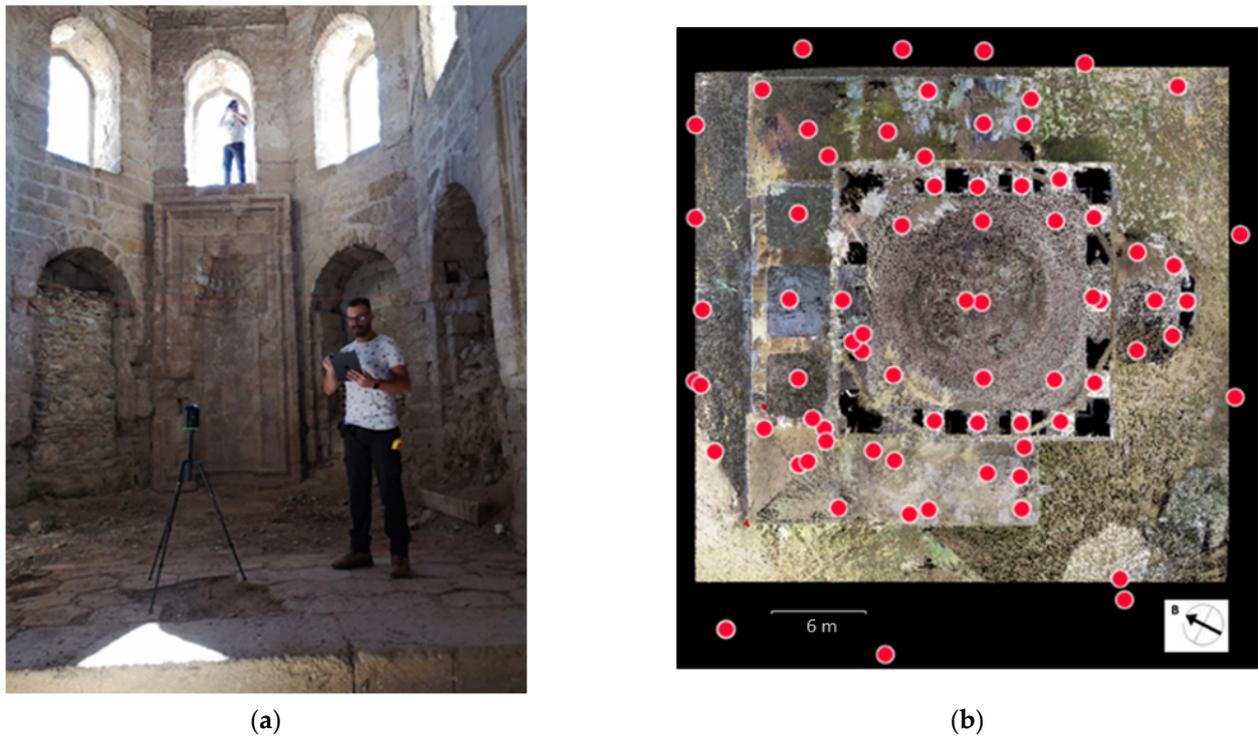
**Figure 10.** Terrestrial laser scanning: (a) data collection in the interior of the monument; (b) laser scanning positions indicated with red dots.
