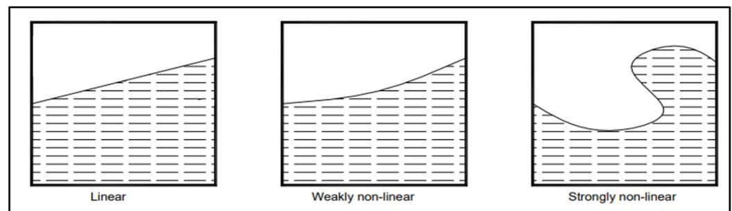
Figure 2. Generic liquid motion types in rectangular containers [18] (p. 6.31).
