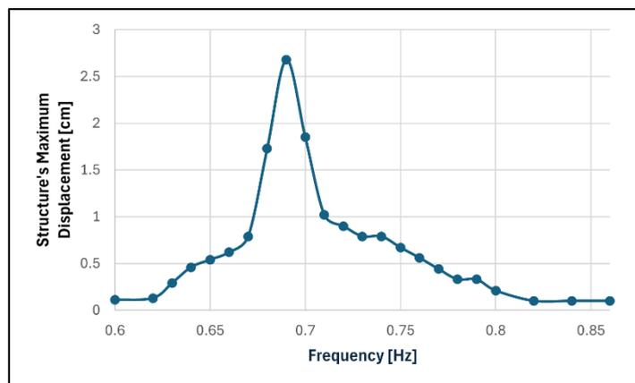
Figure 19. Frequency response of the smaller pendulum without TLD.
