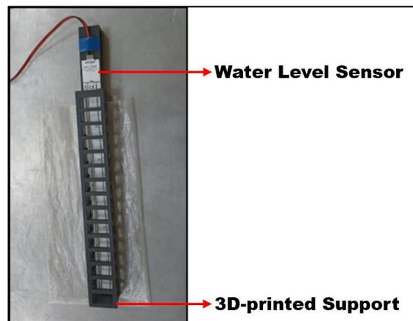
**Figure 14.** Frontal view of the water level sensor with its main components highlighted.
