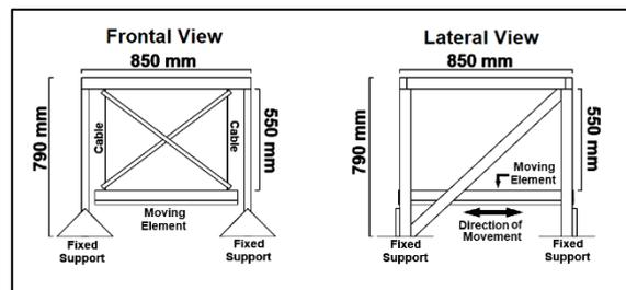
**Figure 4.** Drawings of the frontal (right) and lateral (left) views of the smaller pendulum.
