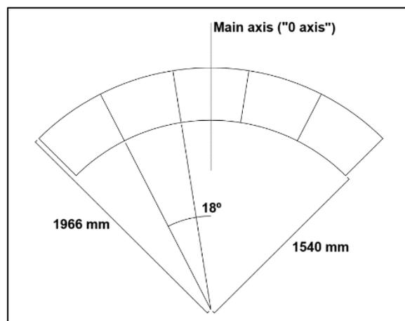
Figure 13. Drawing of the quarter-ring reservoir superior view.
