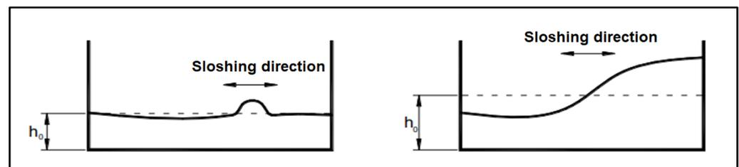
Figure 1. Low (left) and high (right) fill sloshing types in rectangular containers [18] (p. 6.32).
