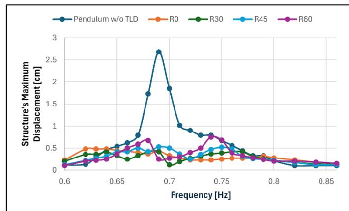
**Figure 21.** Frequency response of the smaller pendulum in configurations R0, R30, R45 and R60 when compared to its response without TLD.**Table 5.** Results of tests with the rectangular TLD on the smaller pendulum.
