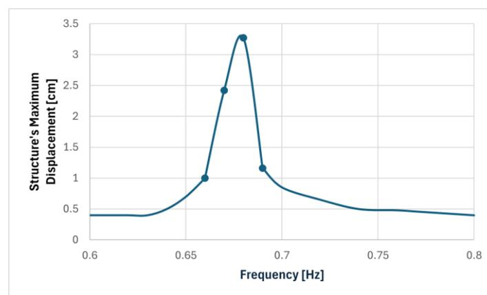
Figure 24. Frequency response of the larger pendulum without TLD.
