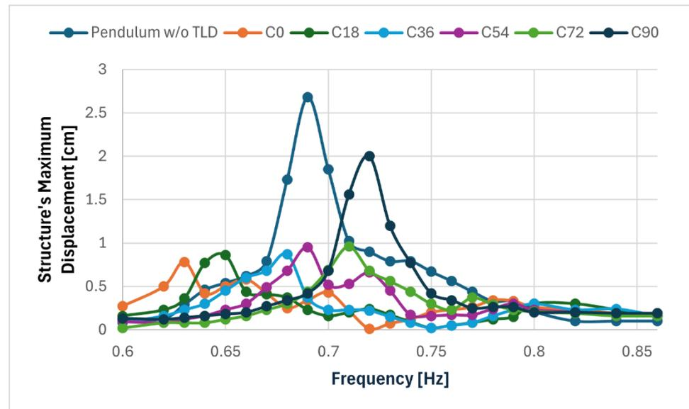
**Figure 23.** Frequency response of the smaller pendulum in configurations C0, C18, C36, C54, C72 and C90 when compared to its response without TLD.
