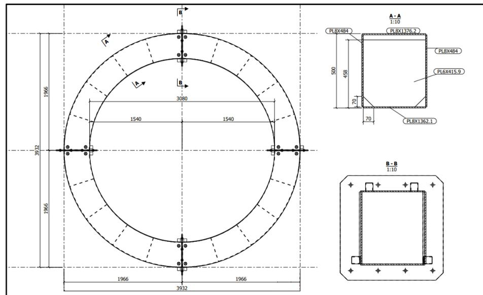
**Figure 9.** Schematics of the annular TLD (top view and two cross-sections).
