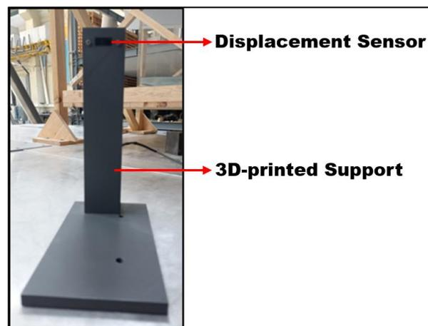
**Figure 15.** Frontal view of the displacement sensor with its main components highlighted.
