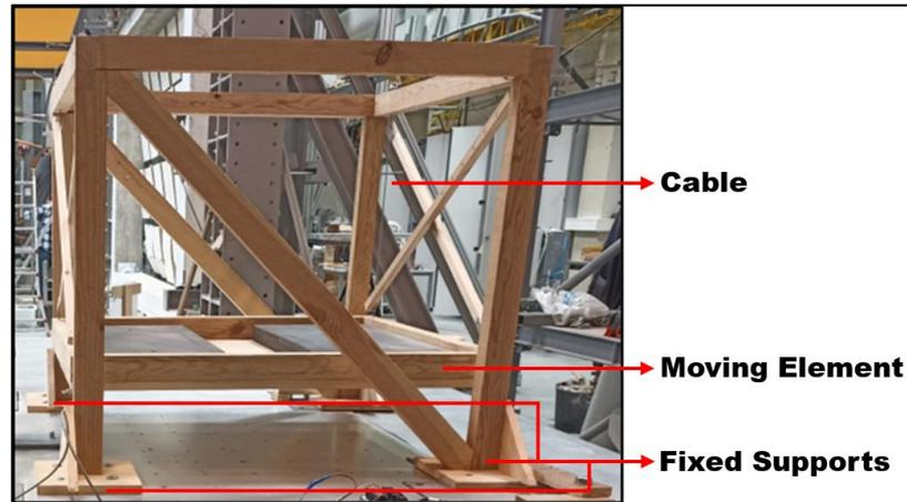
**Figure 3.** Lateral view of the smaller pendulum without any TLD fixed to the shaking table (the 7.15 kg steel plates are not shown in the picture) with its main components highlighted.
