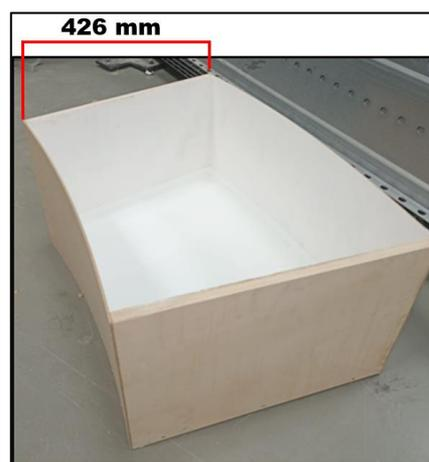
**Figure 10.** A 3/4 superior view of the cell reservoir showing its isolated interior surface, with its length highlighted.
