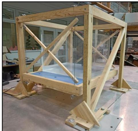
**Figure 20.** Smaller pendulum with the rectangular reservoir in configuration R0.
