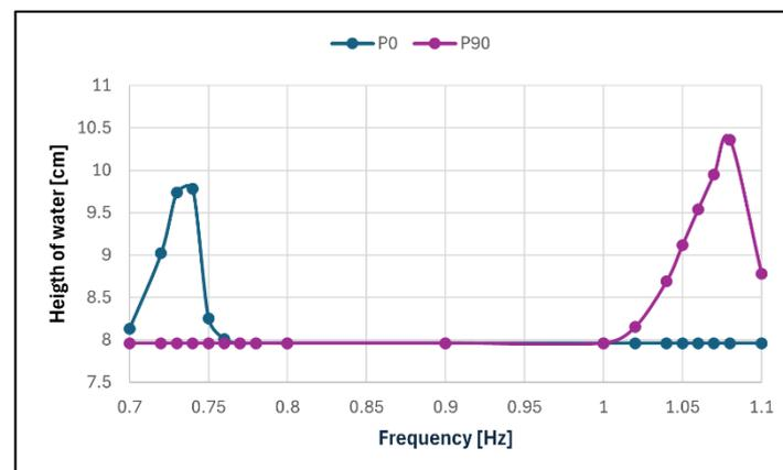
**Figure 17.** Frequency response in configurations P0 and P90.
