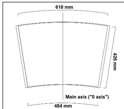
Figure 11. Drawing of the cell reservoir superior view.
