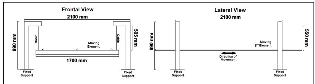
**Figure 6.** Drawings of the frontal (right) and lateral (left) views of the larger pendulum (without the “mass”).
