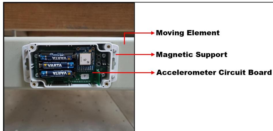
**Figure 16.** Frontal view of the accelerometer (showing its circuit board) fixed to the larger pendulum moving element by its magnetic support.
