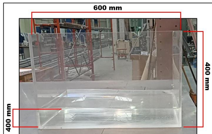
**Figure 7.** Lateral view of the rectangular reservoir filled with water (with a height of 10 cm) with its dimensions highlighted.
