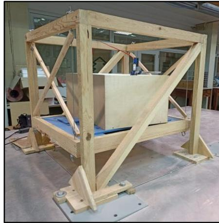
**Figure 22.** Smaller pendulum with the ring cell reservoir in configuration C0.
