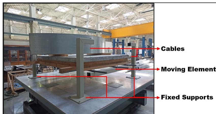
**Figure 5.** 3/4 view of the larger pendulum fixed to the shaking table (the quarter-ring TLD is installed on the pendulum) with its main components highlighted.
