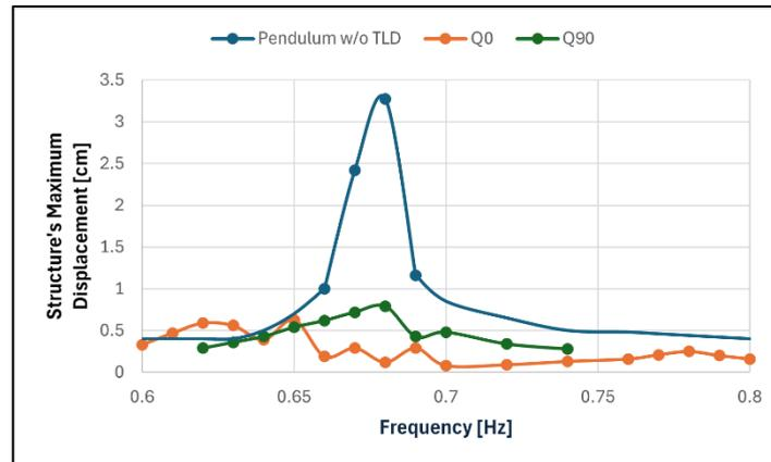
Figure 26. Frequency response of the larger pendulum in configurations Q0 and Q90 when compared to its response without TLD.
