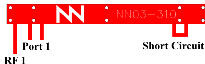
Figure 2. A 30 \text{ mm} \times 3 \text{ mm} \times 1 \text{ mm} antenna booster element with 1 RF port and 1 filtering port; RF2 is unconnected and Port 2 is short-circuited.
