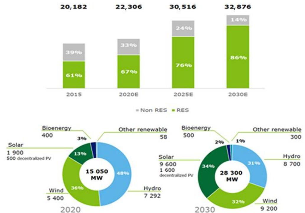
**Figure 2.** Evolution (top) and distribution (bottom) of installed capacity by RES in Portugal (MW).
