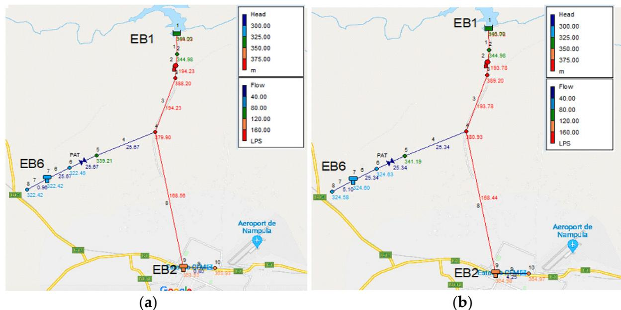
Figure 15. PAT application: (a) results at 3.00 a.m.; (b) results at 11.00 a.m.
