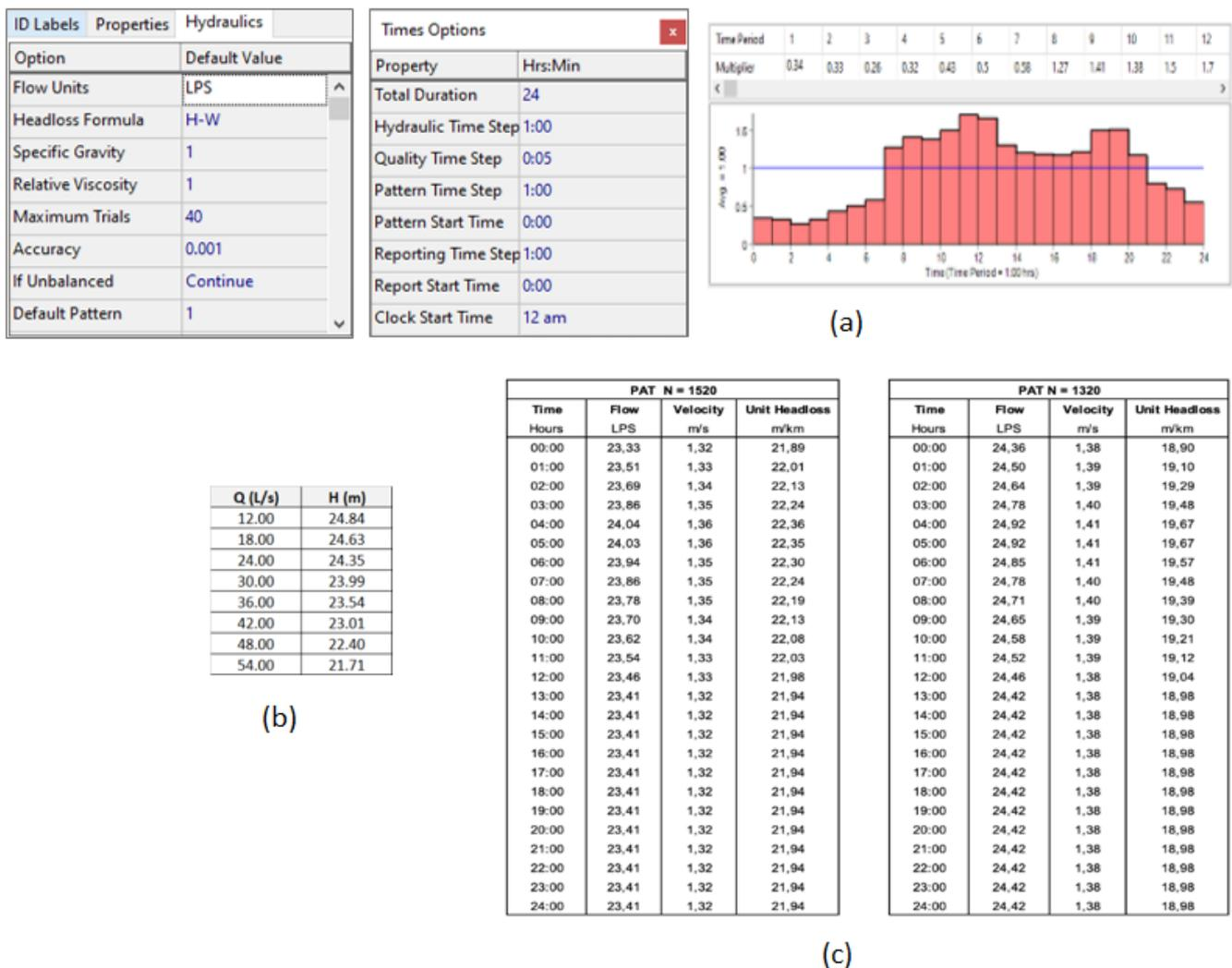
Figure 13. Hydraulic and time characteristics and demand pattern (a), characteristic curve (CCI) based on EPANET simulations (b), and the system behaviour over 24 h for different rotational speeds of the selected PAT (c).
