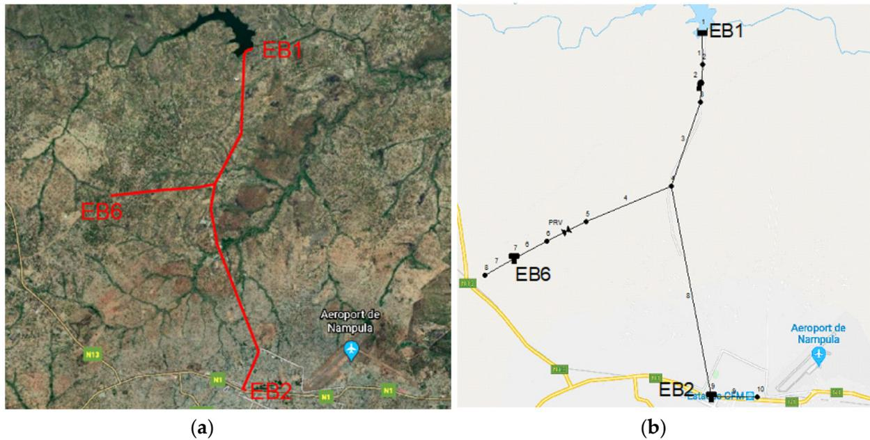
Figure 11. Nampula WSS: (a) implantation area; (b) EPANET model.
