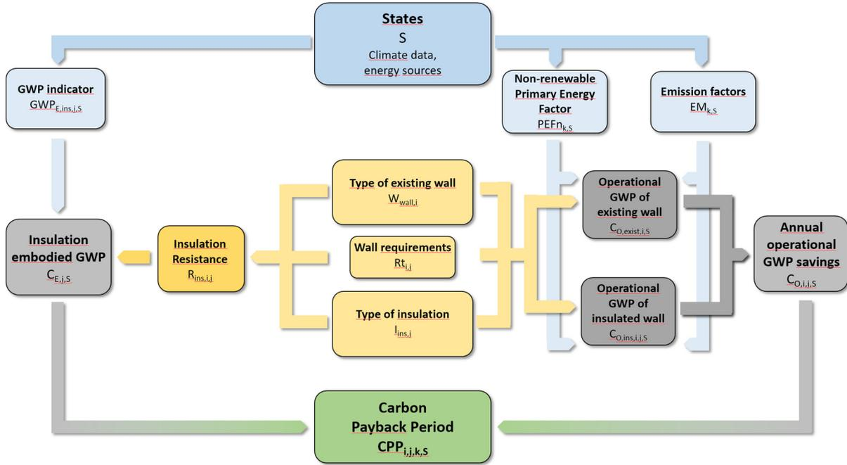
**Figure 2.** Scheme of the CPP calculation methodology.
