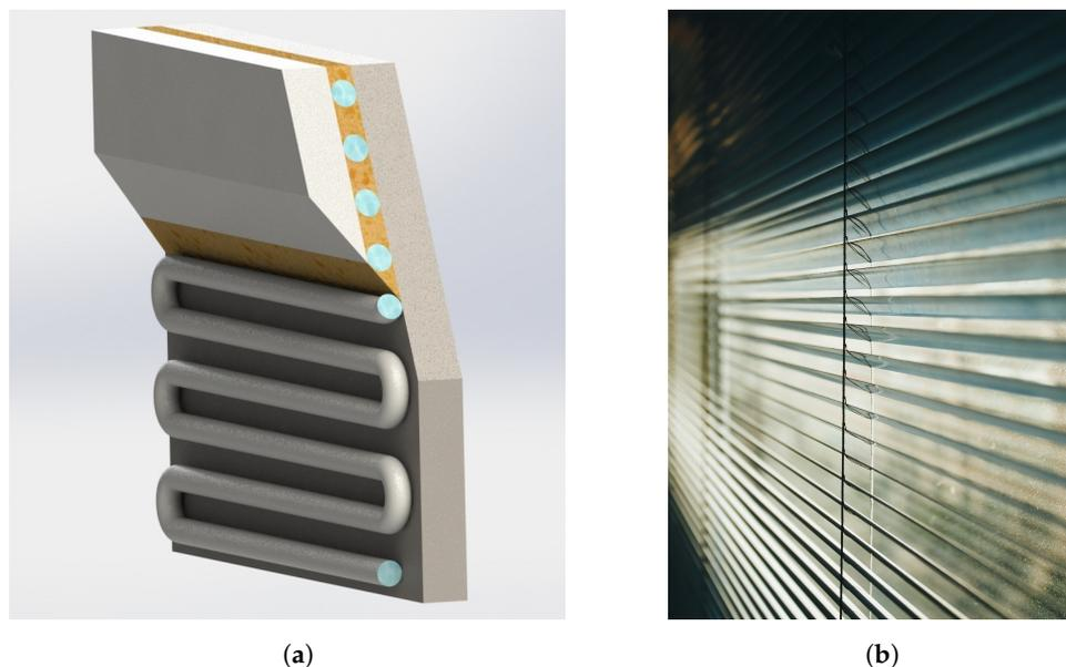
**Figure 3.** (a) Pipe-embedded insulation controls heat transfer within the building envelope by modulating the fluid flow within pipes using pumps and valves. Image redrawn from [37]. (b) Topology morphing insulation adapts its shape to regulate heat transfer. This image showcases Venetian blinds, a prevalent type of window covering that effectively limits radiative heat transfer. Image courtesy of Ave Calvar Martinez, via Pexels, licensed using Pexels License [38].
