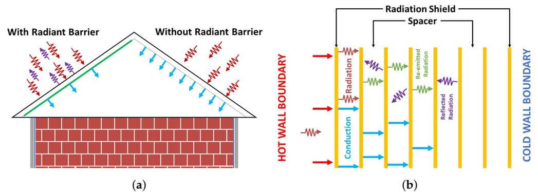
**Figure 11.** (a) Example of a radiant barrier applied under roofing. (b) Cross-section of a multi-layer insulation system, showcasing the arrangement of low-emissivity coatings and radiant barriers for effective heat transfer reduction. Image redrawn from [128].
