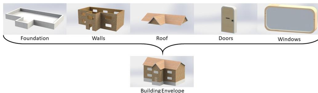
**Figure 1.** The building envelope, comprising the opaque and translucent components, acts as a barrier between the building’s interior and the external environment. The opaque envelope encompasses the walls, roofs, floors, and doors, while the translucent envelope comprises elements such as windows.
