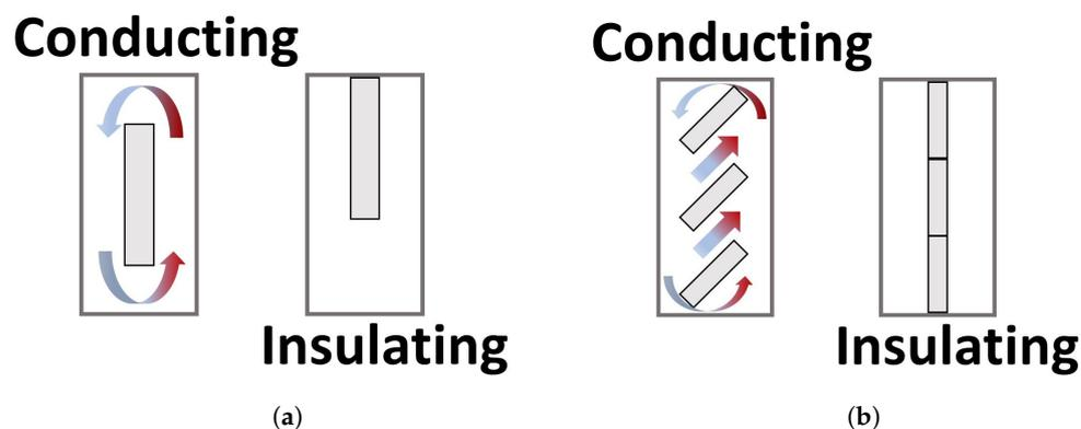
**Figure 9.** Images showcasing innovative design elements that promote or inhibit convection through (a) translation and (b) rotation mechanisms for enhanced heat transfer control. Images respectively redrawn from [98,100].
