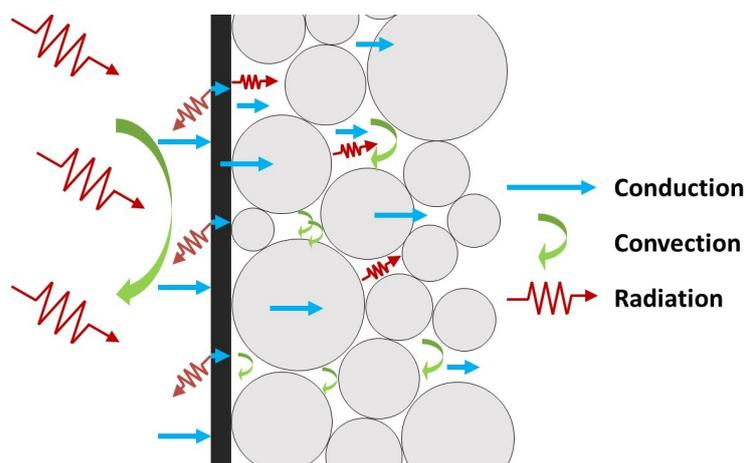
**Figure 4.** In porous insulation materials such as cellulose, heat conduction occurs through two distinct pathways: one that directly traverses the material itself, and another that transfers heat into the material through its pores. Image redrawn from [39].
