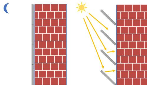
**Figure 12.** An image showcasing a dynamic surface design that regulates radiative heat transfer by selectively concealing and revealing elements with high absorptivity and reflectivity properties. Adapted from [129] and research by Burdajewicz et al. [130].
