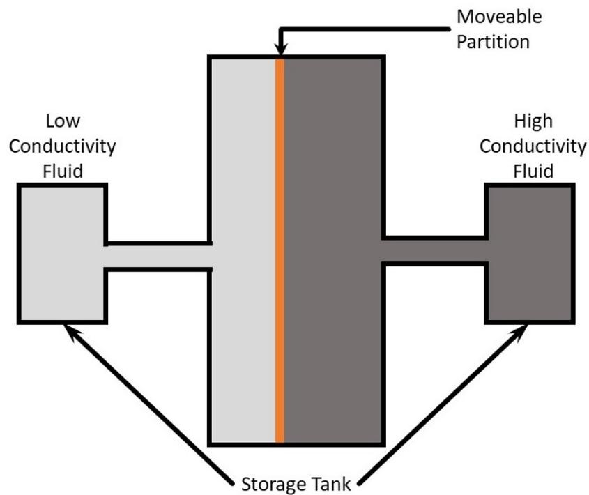
**Figure 5.** By adjusting the thermal conductivity of the fluid by either changing the fluid itself or manipulating its properties, it becomes possible to regulate the heat transfer through the insulation. Redrawn from [56].
