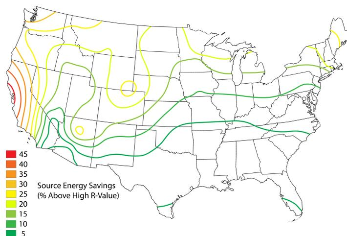
**Figure 2.** Contour map showing the percentage of energy savings when using dynamic insulation with properties that can be controlled. The contours showing the total energy savings of dynamic insulation are calculated with respect to static insulation with the highest recommended R-value mandated by local building codes or regulations. Image redrawn from [35].
