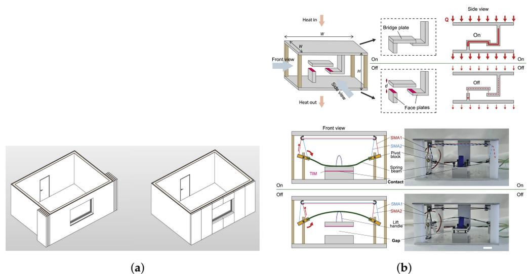
**Figure 6.** (a) Large moveable panels of insulation designed for storage and motion, illustrating their potential for adaptive thermal regulation in building envelopes. Reprinted from [58], licensed under CC-BY-3.0. (b) Precise control with minimal mass displacement through small moveable insulation. Reprinted from [59], licensed under CC-BY-NC-ND-4.0.
