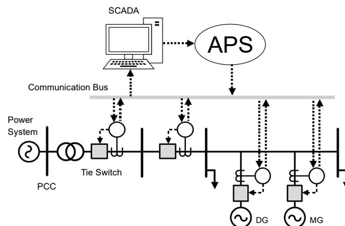
**Figure 1.** Architecture of the proposed APS.
