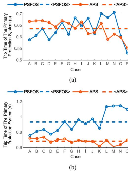
**Figure 4.** Average trip times of the primary protection system: (a) grid-connected mode, (b) islanded mode.
