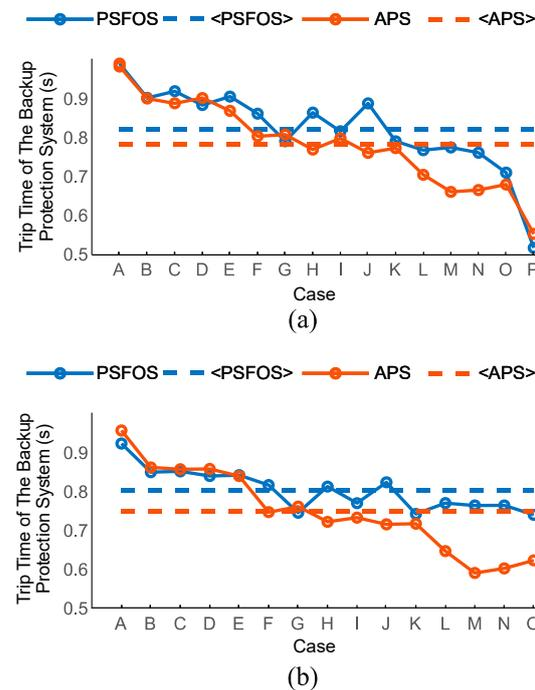
**Figure 5.** Average trip times of the backup protection system: (a) grid-connected mode, (b) islanded mode.
