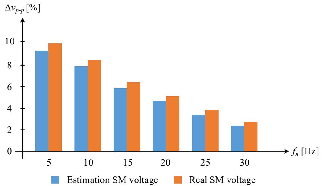
Figure 10. Performance comparison of SM voltage ripple estimation method.
