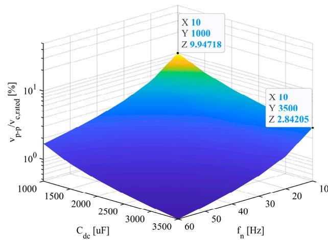
Figure 5. Variation in SM capacitor voltage ripple ( $\Delta v_{p-p}$ ) as influenced by varying capacitance ( $C_{dc}$ ) and operational frequency ( $f_n$ ).
