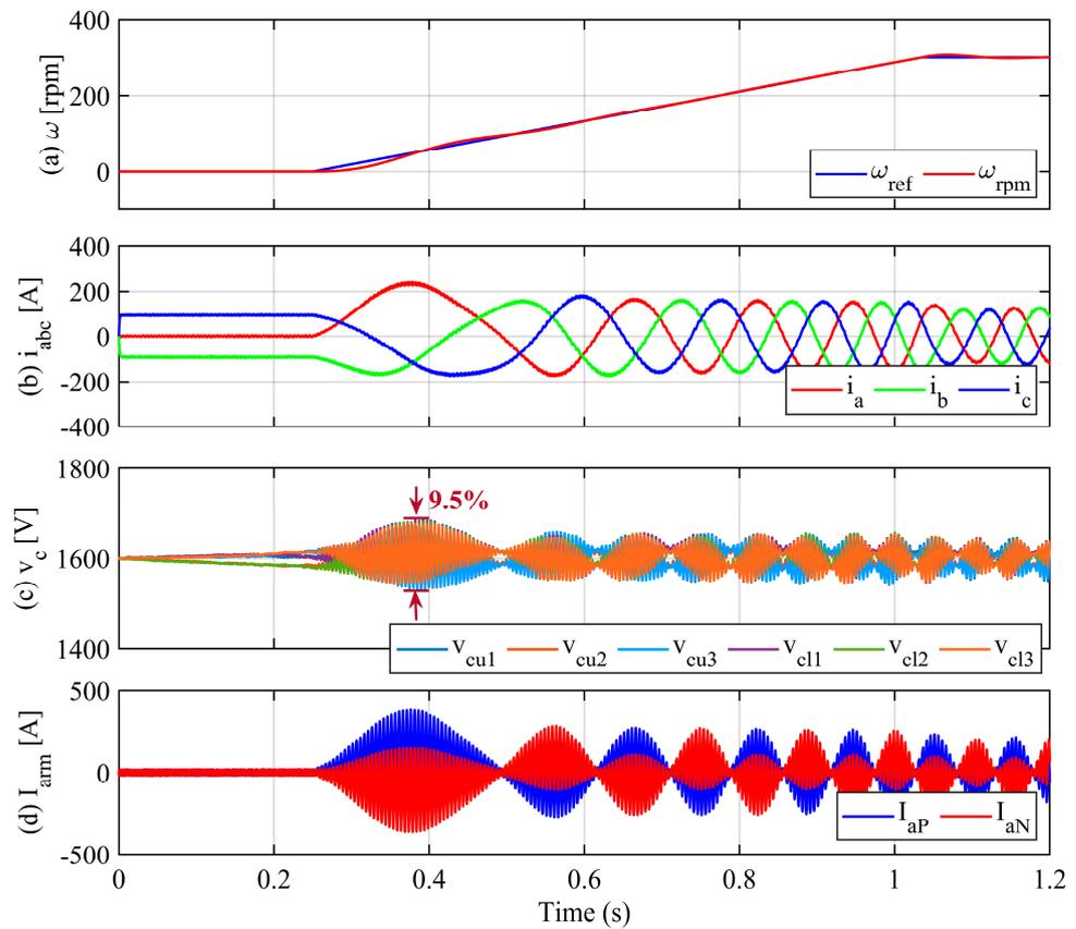
**Figure 12.** Performance of the MMC with proposed SM capacitance selection: (a) motor speed, (b) three-phase current, (c) SM capacitor voltage, (d) arm currents.
