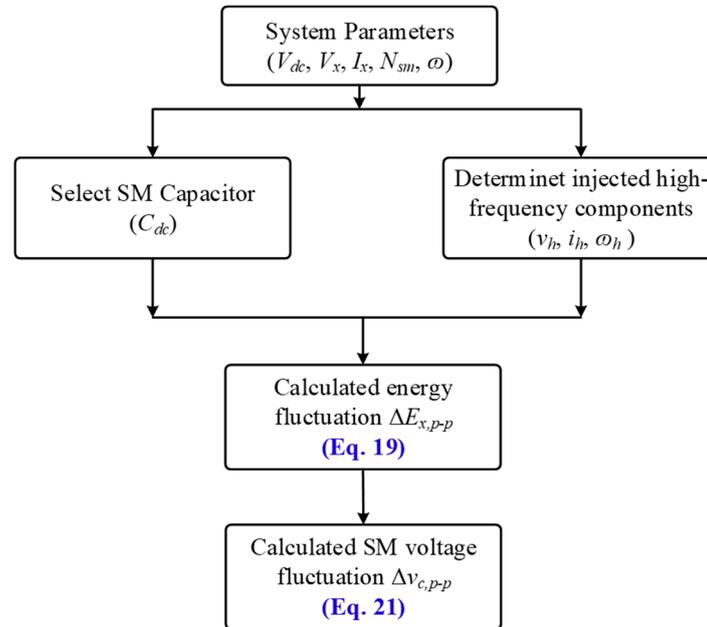
**Figure 3.** Procedure of estimating SM voltage fluctuation ( $\Delta v_{c,p-p}$ ).
