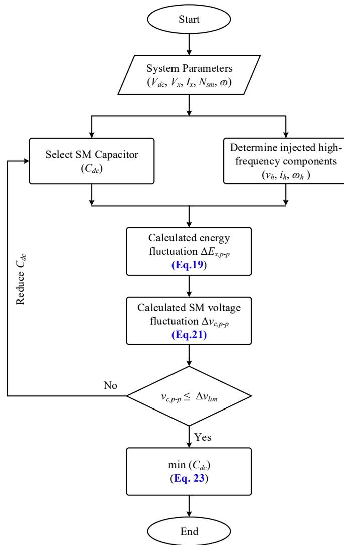
Figure 4. Sizing SM capacitor algorithm.
