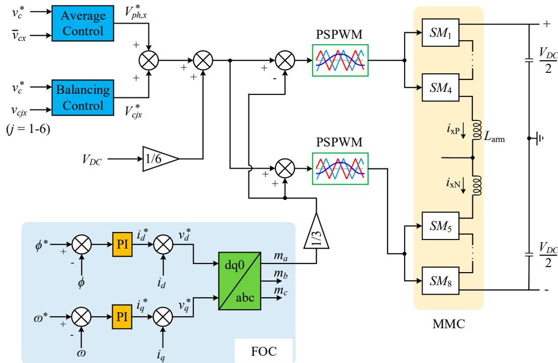
Figure 7. Overall control block diagram of the MMC system.
