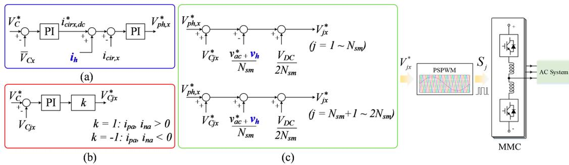
**Figure 6.** SM voltage balancing control based on the high-frequency injection method: (a) phase voltage balancing and circulating current control, (b) individual SM voltage control, (c) SM voltage reference generation.
