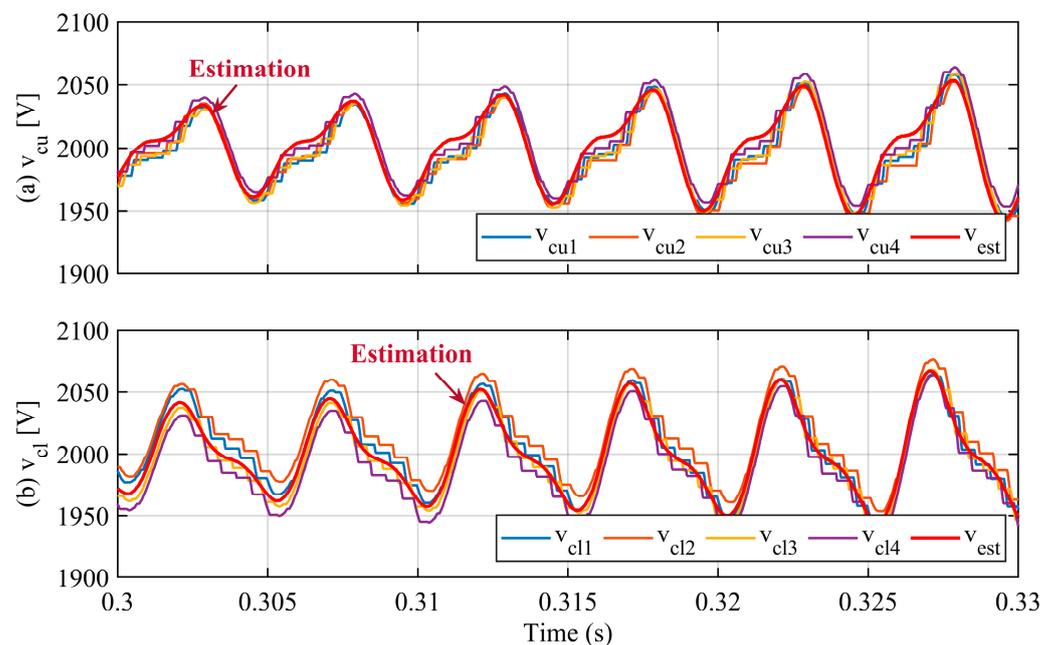
**Figure 9.** The performance of SM voltage estimation algorithm: (a) upper arm SM capacitor voltage, (b) lower arm SM capacitor voltage.
