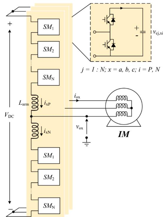
**Figure 1.** Circuit configuration of a three-phase MMC.
