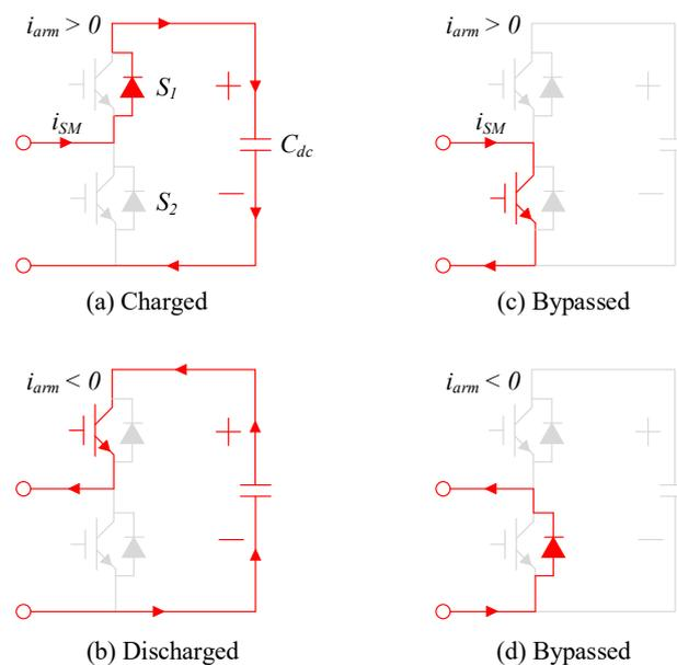
**Figure 2.** The switching state of an HB-SM: (a) charged, (b) discharged, (c,d) bypassed.
