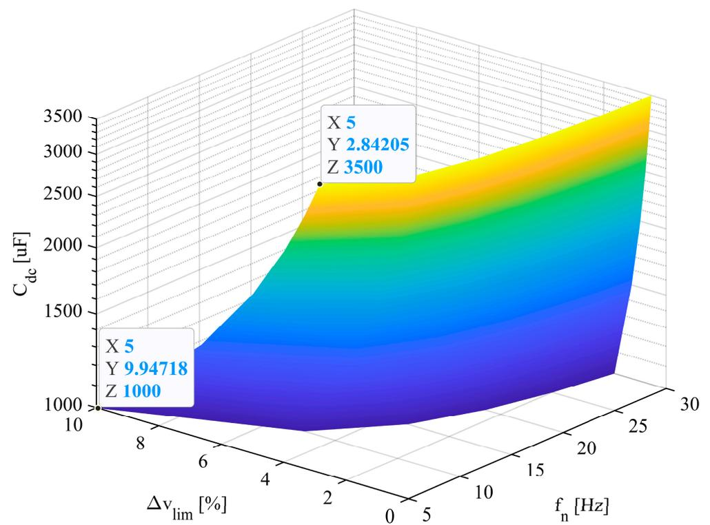
Figure 11. Design of SM capacitance at different operating frequencies based on the predetermined voltage ripple limit ( $\Delta v_{lim}$ ).
