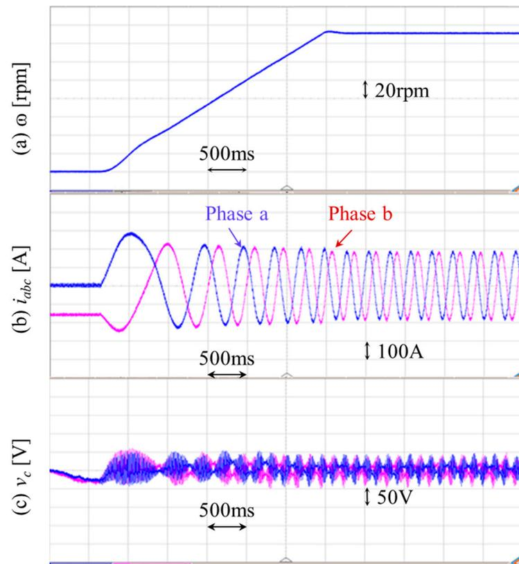
**Figure 15.** Real-time performance of the proposed algorithm: (a) motor speed, (b) output current, (c) SM capacitor voltage.
