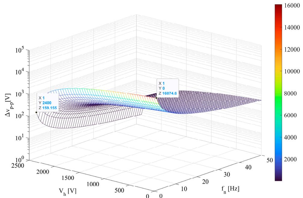
**Figure 8.** Variation in SM capacitor voltage ripple ( $\Delta v_{c,p-p}$ ) based on injected high-frequency components and operating frequency ( $f_n$ ).
