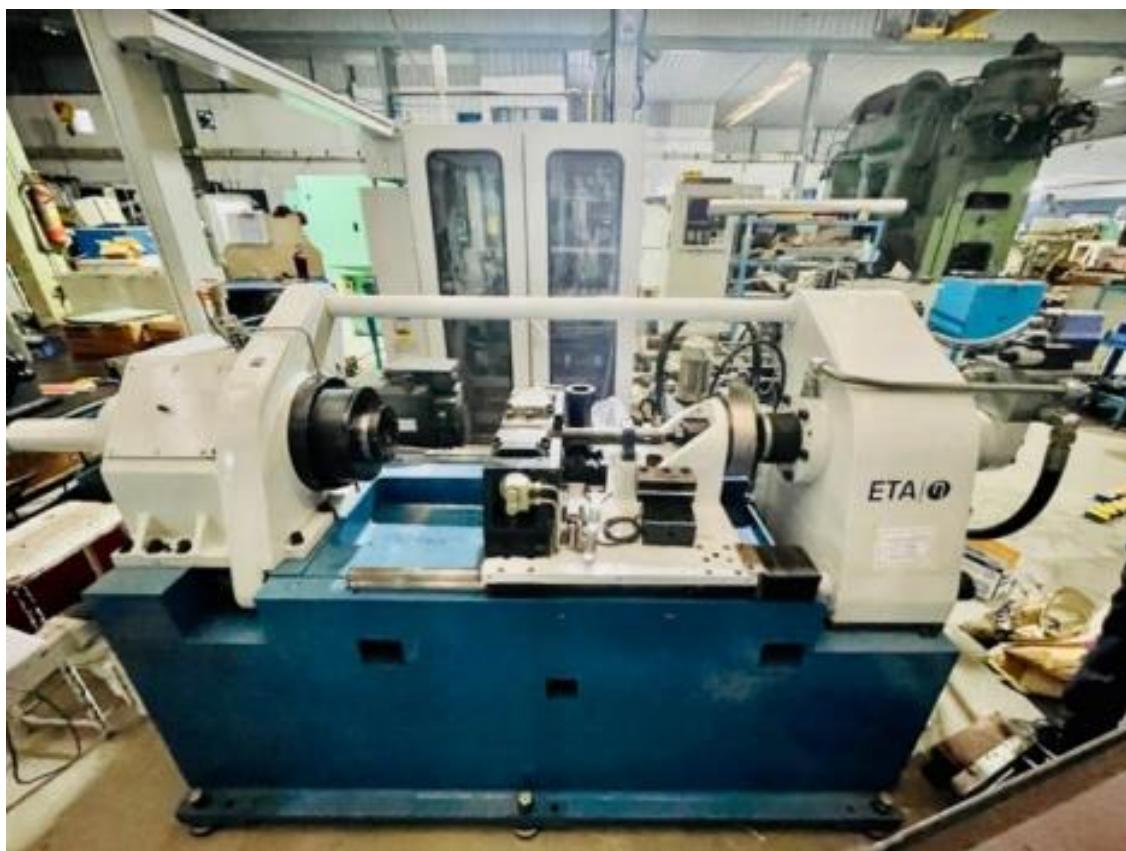
**Figure 1.** Rotary friction welding setup.
