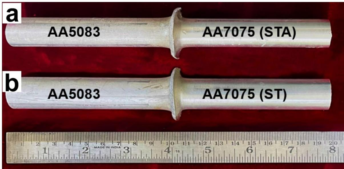
**Figure 5.** Visual view of welded joints (a) AA5083/AA7075-STA and (b) AA5083/AA7075-ST.
