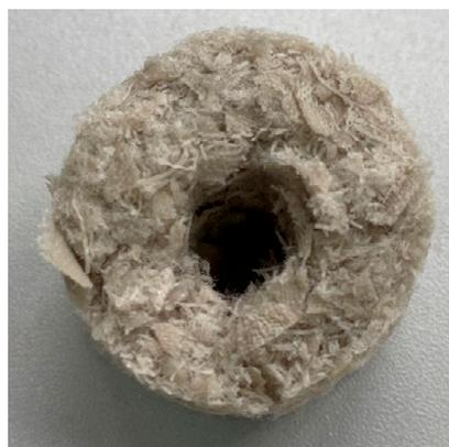
**Figure 16.** Photo of the packing element (green PES).
