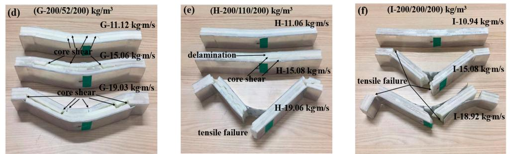
**Figure 7.** The impact force–time curves and failure modes of the sandwich beam with different cores: (a,d) G-200/52/200; (b,e) H-200/110/200; (c,f) I-200/200/200.
