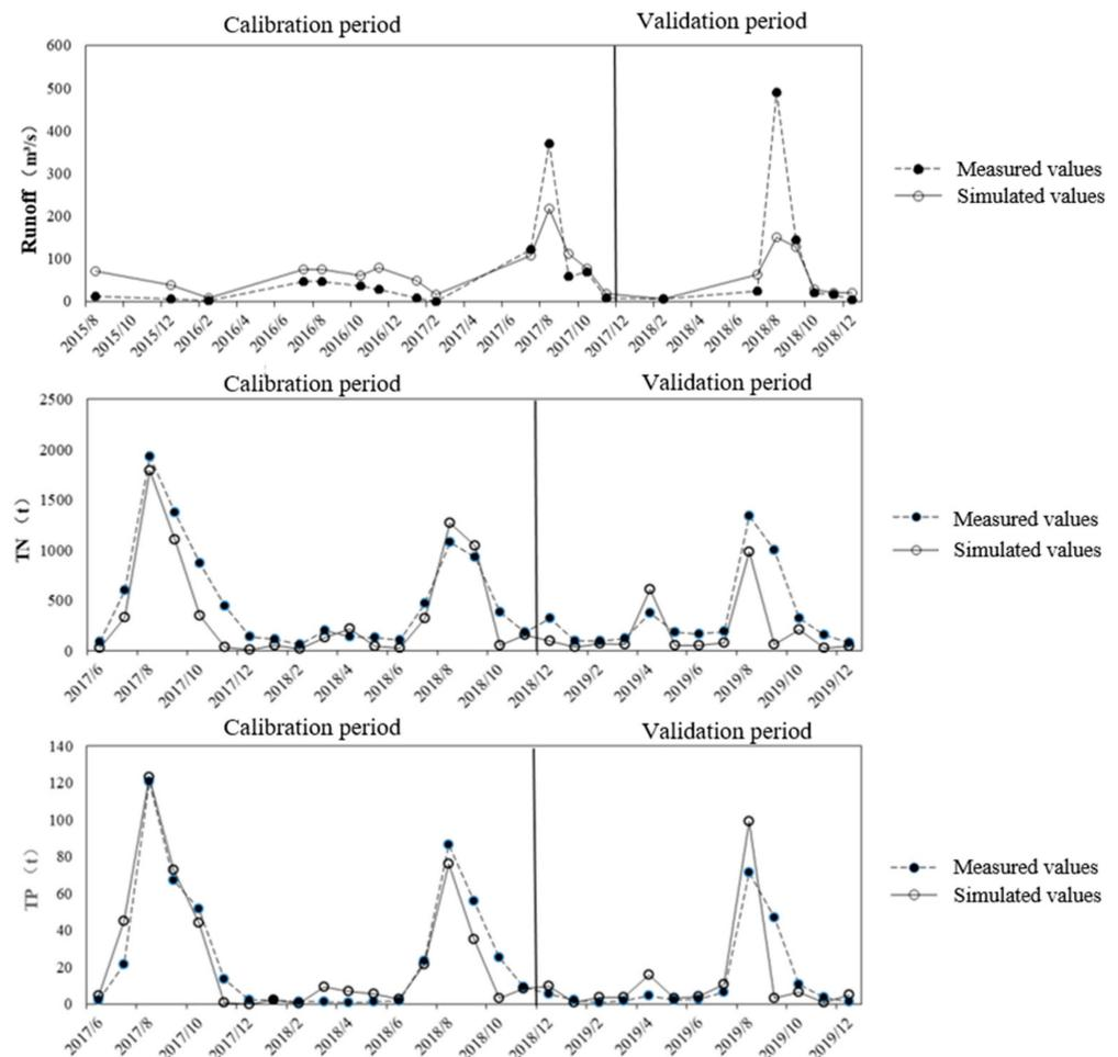
**Figure 3.** Comparison of estimated and measured values of various parameters during the verification period.
