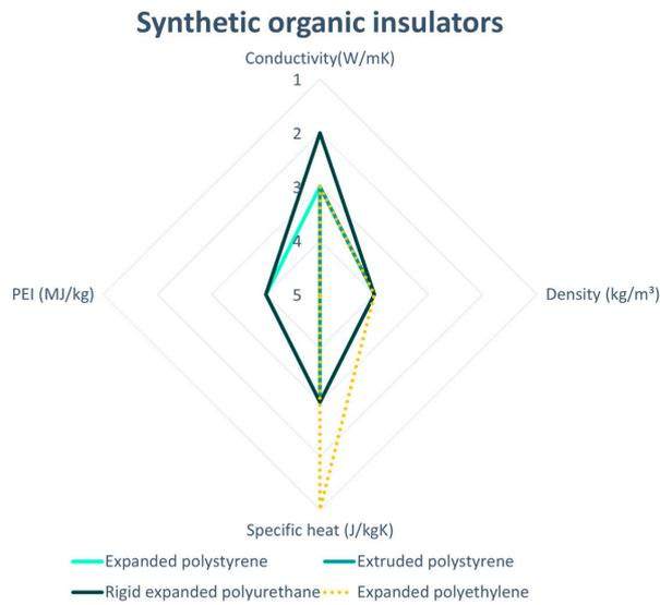
Figure 6. Comparison of synthetic organic insulation materials.
