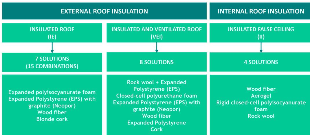
Figure 8. Prefabricated insulation solutions available on the market.
