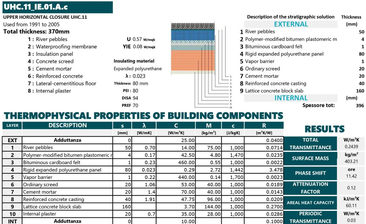
Figure 16. Example of a performance sheet.
