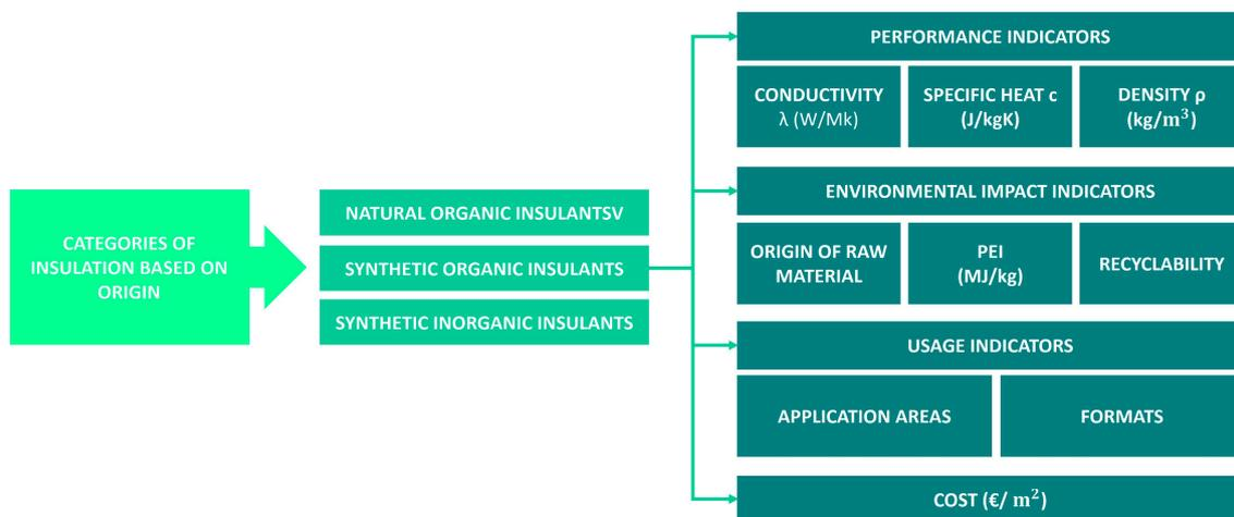
**Figure 4.** Comparison parameters for insulation materials.
