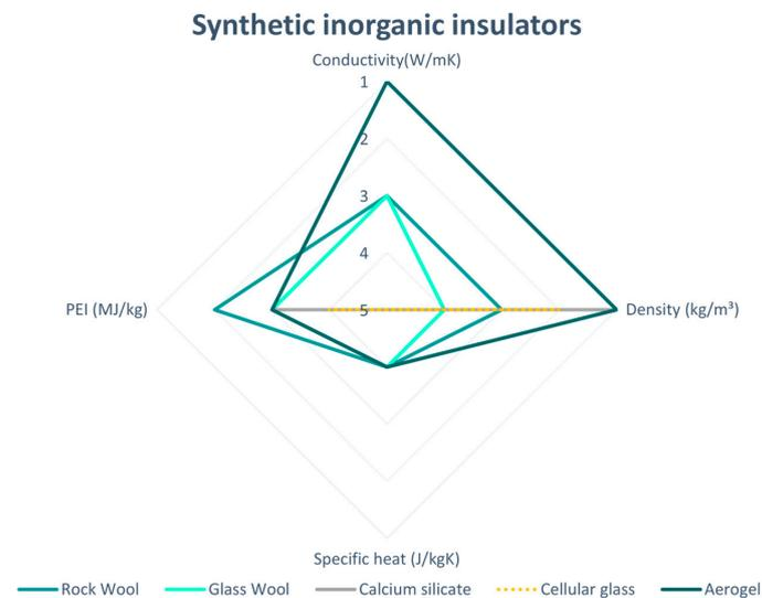
Figure 7. Comparison of synthetic inorganic insulation materials.
