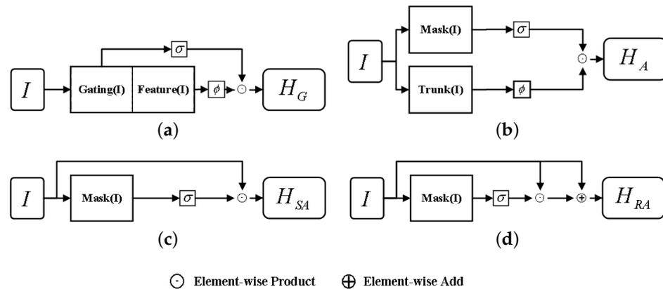
**Figure 2.** Illustration of four modules. The gated convolution could be regarded as a special attention mechanism. (a) Gated convolution. (b) Attention. (c) Self-Attention. (d) Residual attention.
