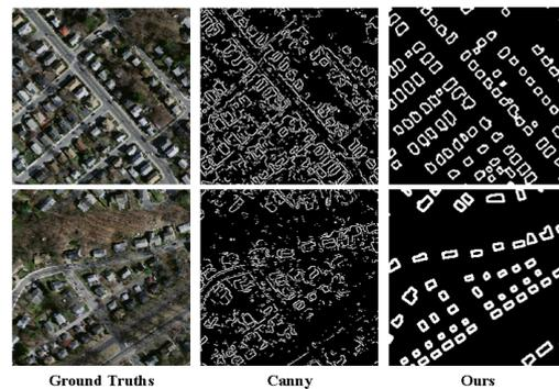
**Figure 7.** Comparison of edge extraction methods. The Canny operator results exhibit many noise points, while ours are significantly clearer and more accurate.
