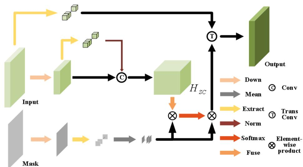
**Figure 3.** The structure of the contextual attention layer. To mitigate the substantial computational burden, this layer resizes the input dimensionality by half while maintaining the original input shape for the output.
