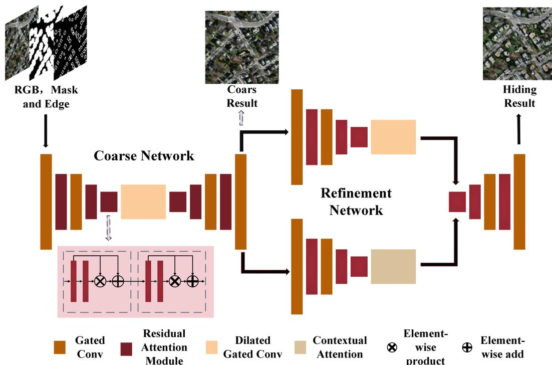
**Figure 1.** The two-stage generator. Refinement Network refines the preliminary inpainting results of the Coarse Network.
