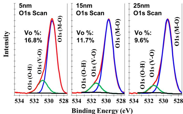
**Figure 3.** XPS spectra of the O 1s signal of a-IGZO film-4 in Table 1 at the detection depths of 5, 15 and 25 nm.
