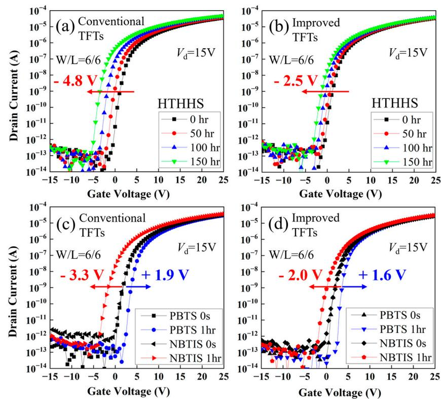
**Figure 4.** (a,b) Evolutions of transfer characteristics of the conventional and improved a-IGZO TFTs under HTHHS conditions. (c,d) Transfer characteristics of conventional and improved a-IGZO TFTs before and after PBTS/NBTIS stress.
