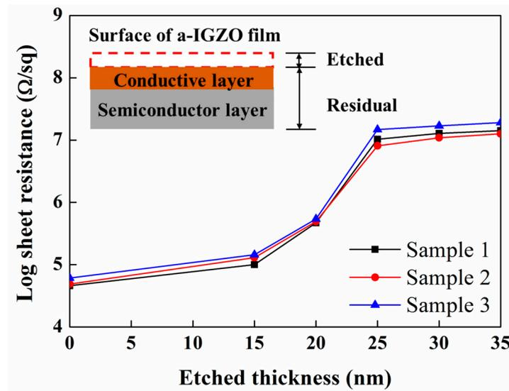
**Figure 2.** The  $R_s$  values of the residual a-IGZO film with various etched thicknesses. The inset shows the schematic cross-section of residual a-IGZO film after being etched in dilute hydrochloric acid. Lines are just to guide the eyes.
