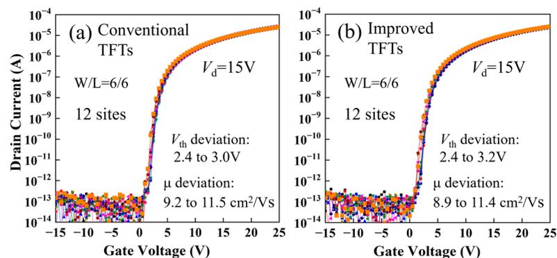
**Figure 5.** The transfer characteristics of the 12 fabricated TFTs on a G4.5 glass substrate, with (a) the conventional TFTs and (b) the improved TFTs.
