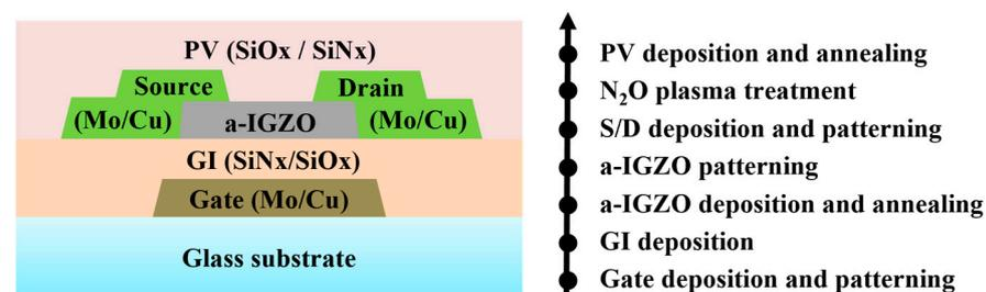
**Figure 1.** The schematic cross-section and the main process flow of the fabricated BCE structured a-IGZO TFTs in this work.
