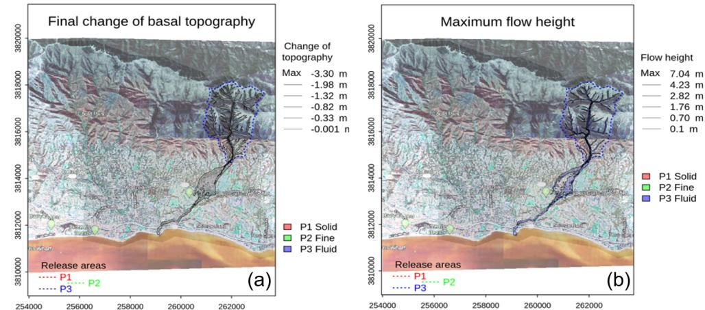
**Figure 12.** (a) Final deposition and (b) maximum flow height at Romero Creek.
