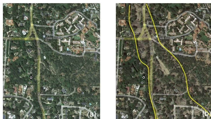
**Figure 6.** Area around Montecito Creek (a) before and (b) after debris flows; the area between the yellow lines highlights the main area affected by the debris flows.
