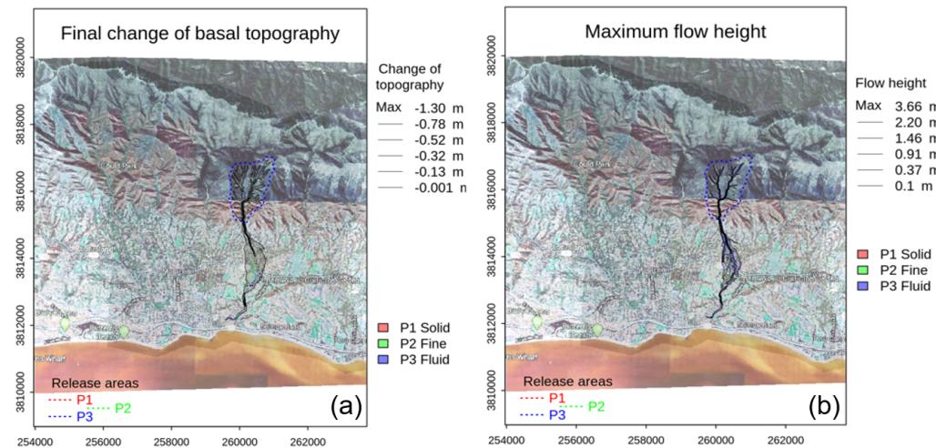
**Figure 11.** (a) Final deposition and (b) maximum flow height at Buena Vista Creek.
