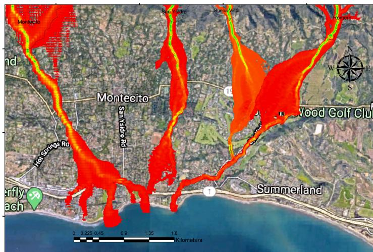
**Figure 13.** Simulation of debris-flow-affected areas; the areas highlighted in red indicate the debris-flow deposits.
