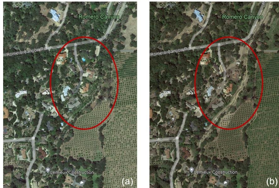
**Figure 8.** Area around Romero Canyon Road (a) before and (b) after the debris flow in Romero Creek; the area circled by the red line indicates the main area affected by the debris flows.
