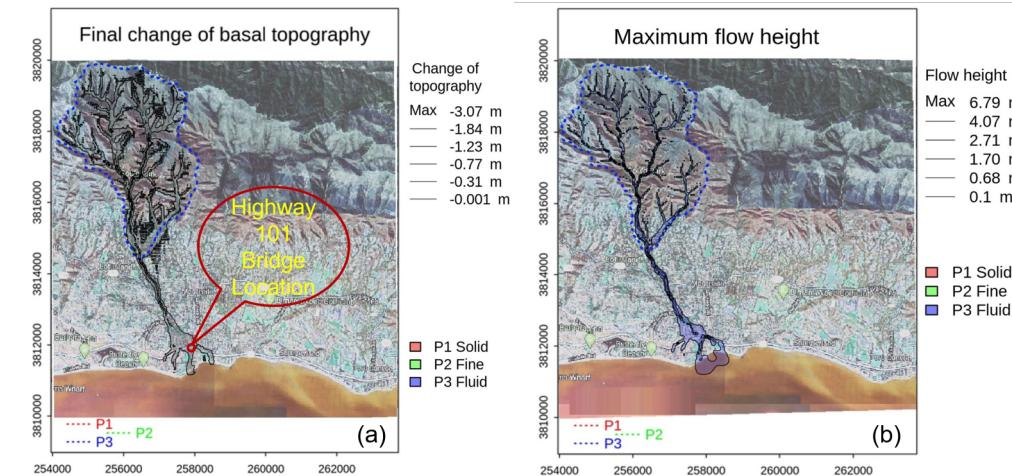
**Figure 9.** (a) Final deposition and (b) maximum flow height at Montecito Creek.
