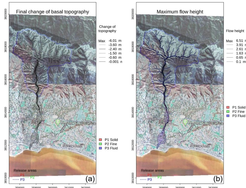
**Figure 10.** (a) Final deposition and (b) maximum flow height at San Ysidro Creek.
