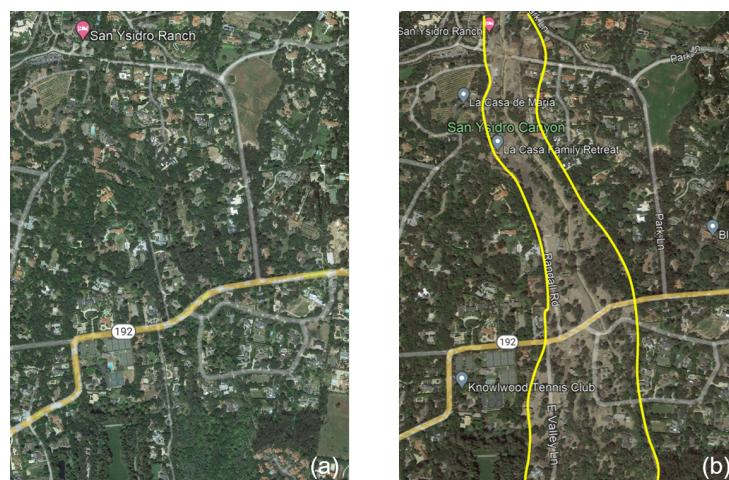
**Figure 7.** Area around the San Ysidro Creek (a) before and (b) after debris flows around Highway 192 in Montecito; the area between the yellow lines highlights the main area affected by the debris flows.
