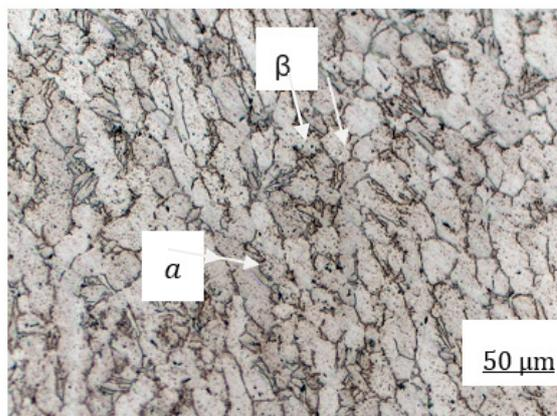
**Figure 2.** Optical micrographs showing the microstructure of Ti-6Al-4V alloy.
