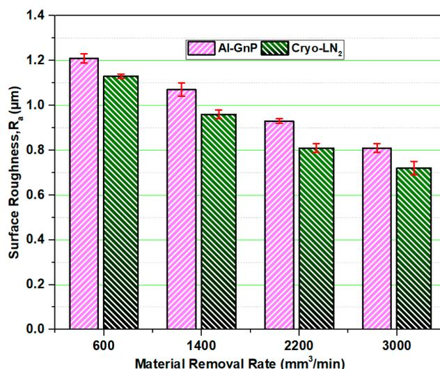
**Figure 9.** Comparison of the surface quality of workpieces under hybrid nanofluid- and cryogenic LN<sub>2</sub>-assisted machining processes ( $a_p = 0.8$  mm;  $f = 0.1$  mm/rev;  $P = 0.5$  MPa;  $n_p = 1.2$ ).
