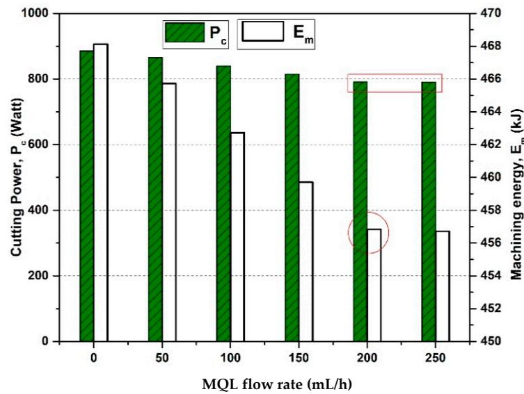
**Figure 5.** Effect of minimum quantity lubrication (MQL) flow rate on power and energy consumption ( $v_c = 70$  m/min,  $a_p = 0.8$  mm;  $f = 0.1$  mm/rev;  $P_p = 0.5$  MPa).
