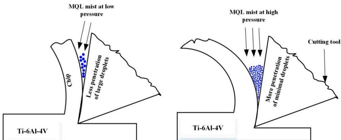
Figure 7. Effect of air pressure on airdrops at the machining zone.
