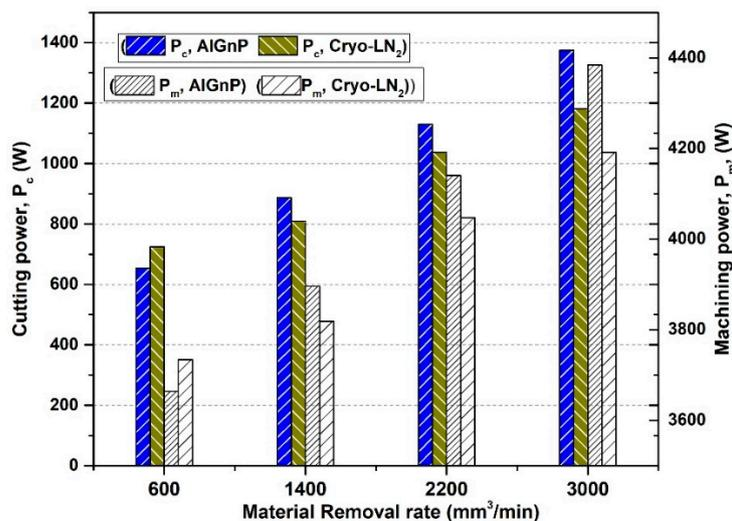
**Figure 10.** Effect of increasing material removal rate (MRR) on cutting power and machining energy in Al-GnP-assisted machining and cryogenic LN<sub>2</sub>-assisted machining ( $a_p = 0.8$  mm;  $f = 0.1$  mm/rev;  $P = 0.5$  MPa;  $n_p = 1.2$ ).
