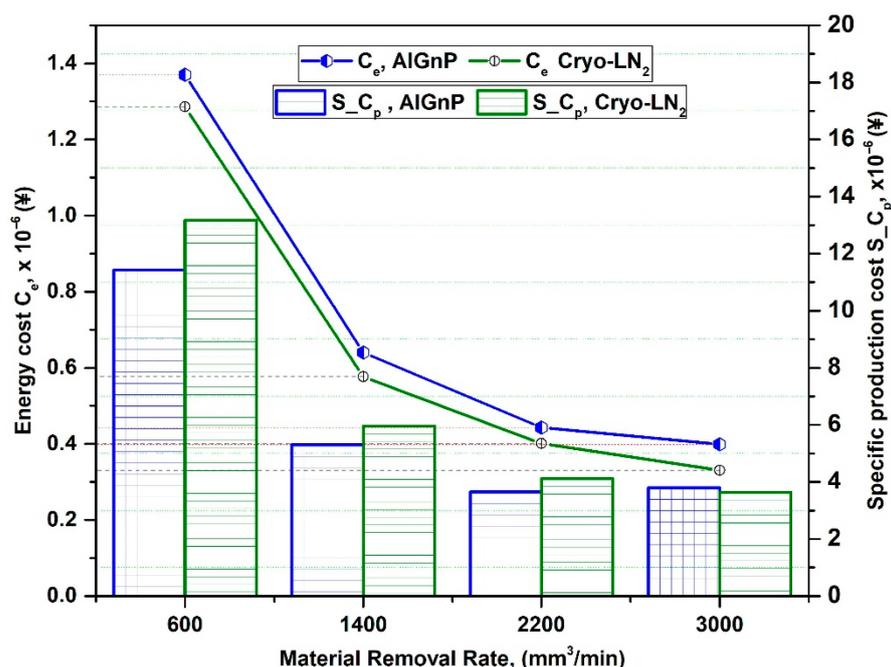
**Figure 13.** Comparison of energy cost and specific production cost under two various cooling/lubrication approaches ( $a_p = 0.2$  mm;  $f = 0.1$  mm/rev;  $p = 0.5$  MPa;  $n_p = 1.2$ ).
