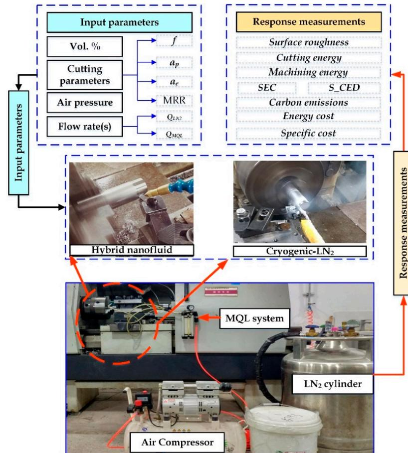
**Figure 3.** Experimental setup for hybrid nanofluid and cryogenic  $\text{LN}_2$  approaches.
