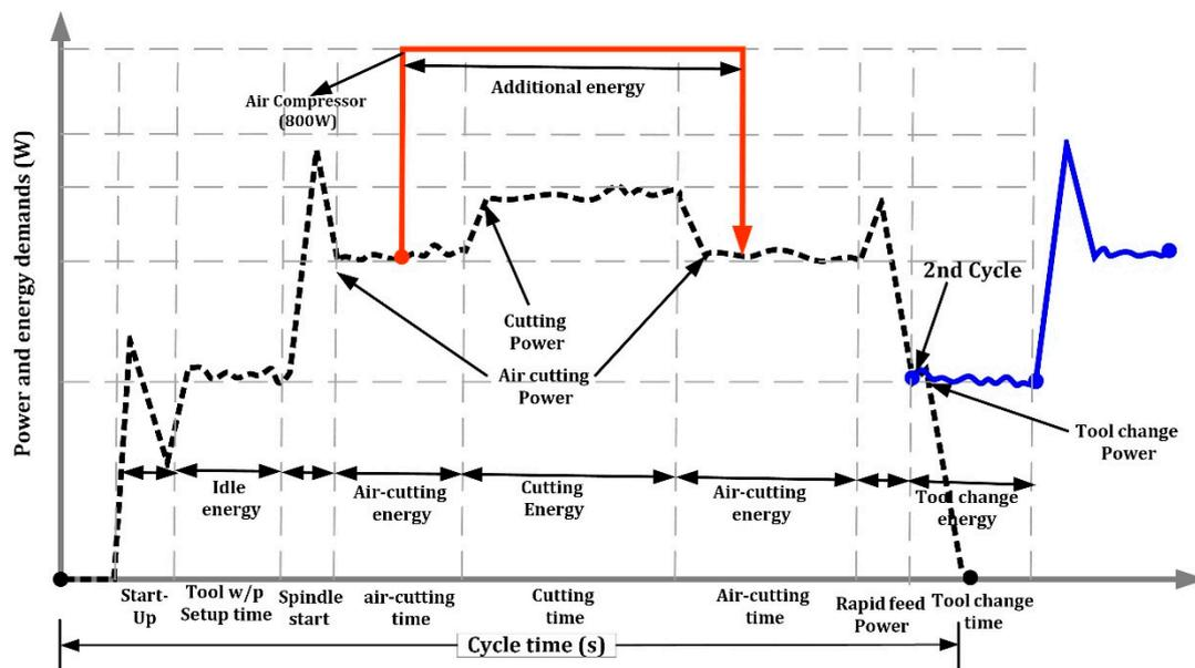
Figure 1. Power and energy consumption in various functionality states of machine tool.
