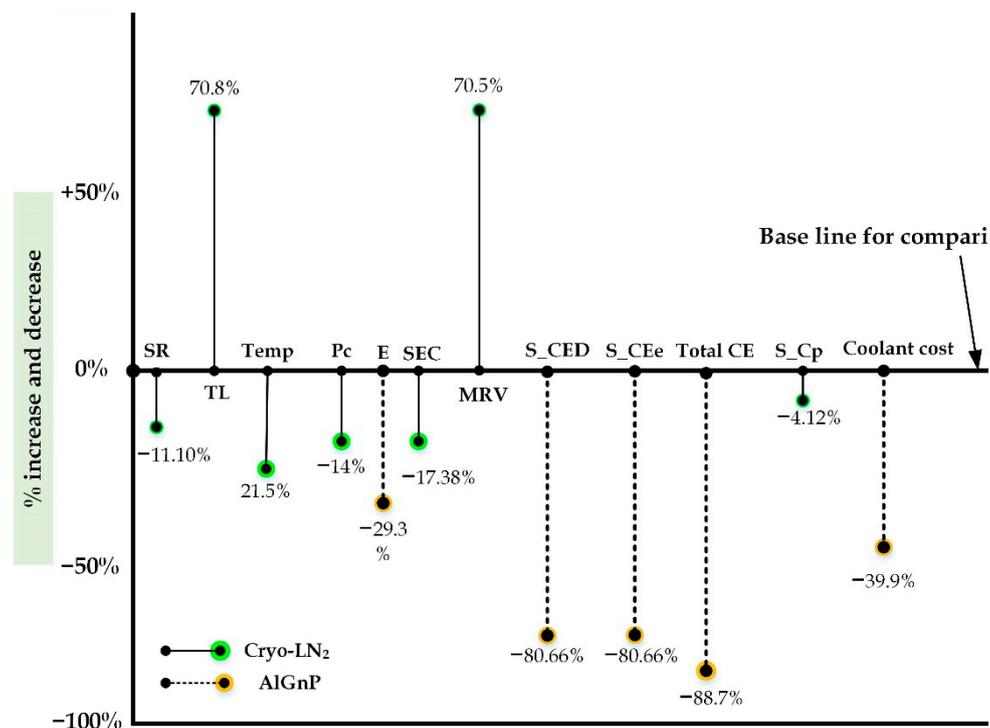
**Figure 14.** A holistic comparison between hybrid Al-GnP and cryogenic LN<sub>2</sub> at higher cutting conditions ( $a_p = 0.8$  mm;  $f = 0.1$  mm/rev;  $P = 0.5$  MPa;  $v_c = 150$  m/min).
