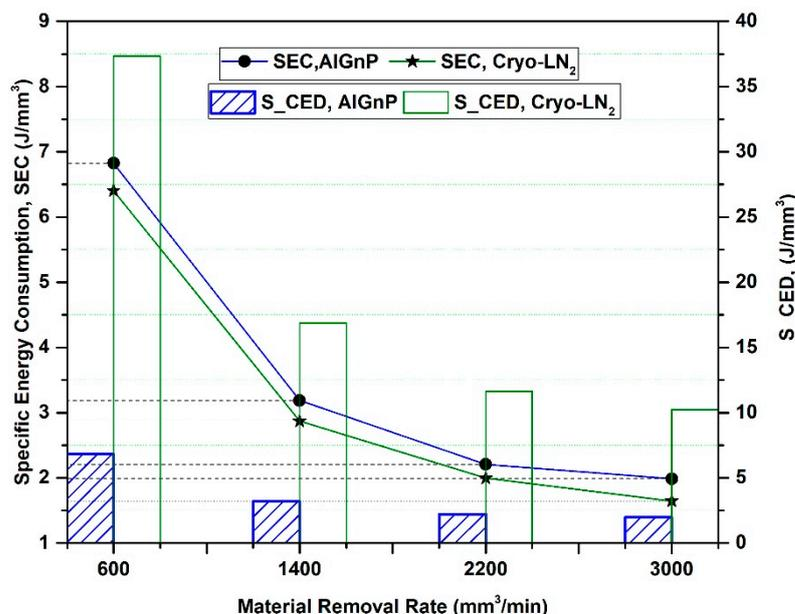
**Figure 11.** Influence of *MRR* on specific energy consumption (SEC) and specific cumulative energy demand (*S\_CED*) under both environments ( $a_p = 0.8$  mm;  $f = 0.1$  mm/rev;  $P = 0.5$  MPa;  $n_p = 1.2$ ).
