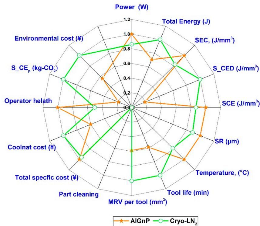
**Figure 15.** Radar graph to evaluate overall process performance ( $a_p = 0.8$  mm;  $f = 0.1$  mm/rev;  $P = 0.5$  MPa;  $v_c = 150$  m/min).
