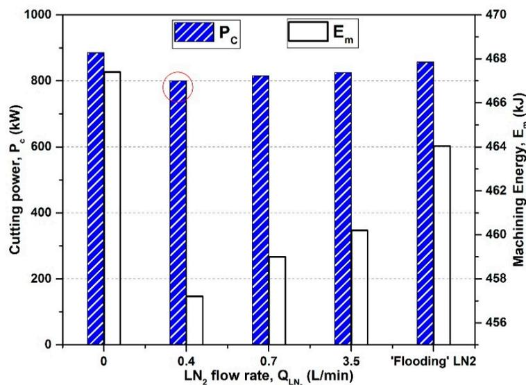
**Figure 4.** Influence of LN<sub>2</sub> flow rate on cutting power and machining energy ( $v_c = 70$  m/min,  $a_p = 0.8$  mm;  $f = 0.1$  mm/rev).
