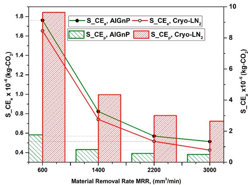
**Figure 12.** Influence of *MRR* on carbon footprint of electrical energy consumption and CO<sub>2</sub> emissions per part ( $a_p = 0.8$  mm;  $f = 0.1$  mm/rev;  $p = 0.5$  MPa;  $n_p = 1.2$ ).
