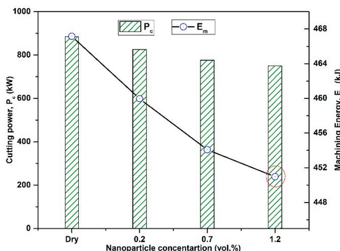
Figure 8. Effect of nanoparticles' concentration on sustainable indicators ( $a_p = 0.8$  mm;  $f = 0.1$  mm/rev;  $P = 0.5$  MPa).
