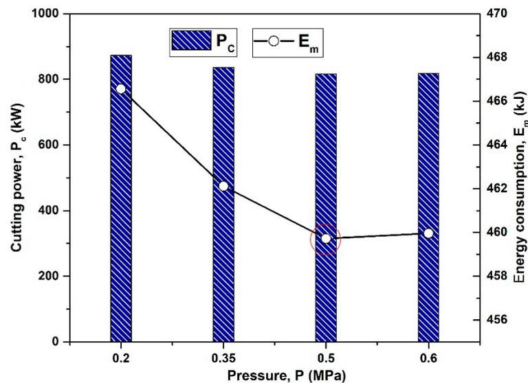
**Figure 6.** Effect of mist pressure on energy and power consumption ( $v_c = 70$  m/min,  $a_p = 0.8$  mm;  $f = 0.1$  mm/rev;  $n_p = 1.2$ ).
