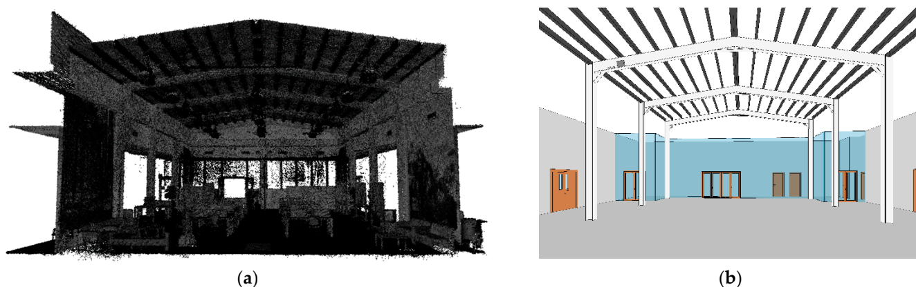
Figure 5. Monitored gable frame: (a) cloud points model; (b) BIM model in Revit.
