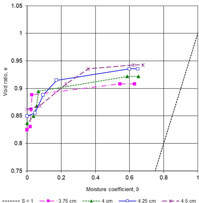
**Figure 3.** Reinterpretation of the results of the wetting test of a Vertisol sample with an initial height of 6.2 cm, performed by Garnier et al. [23] (swelling curves interpreted at different levels of the test sample during the wetting test).
