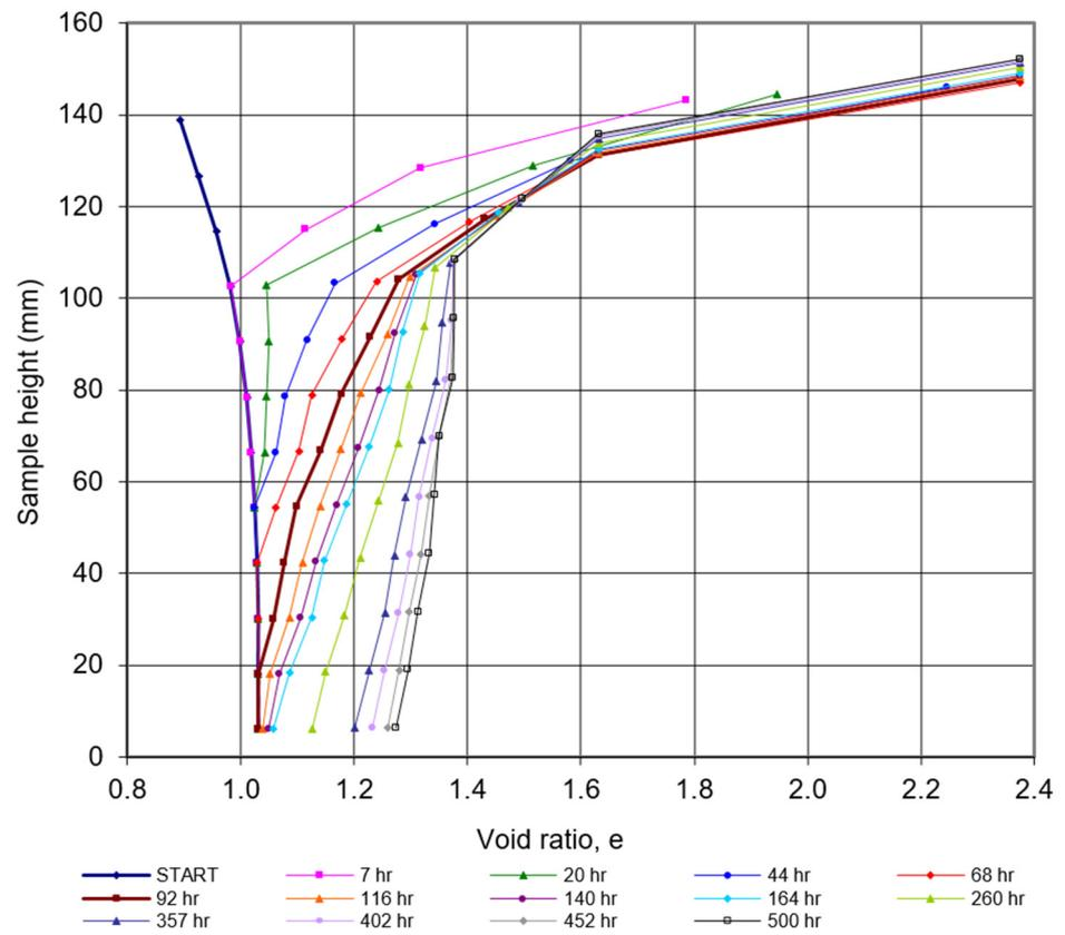
Figure 10. Profiles of the void ratio in the wetting experiment of VU-3.
