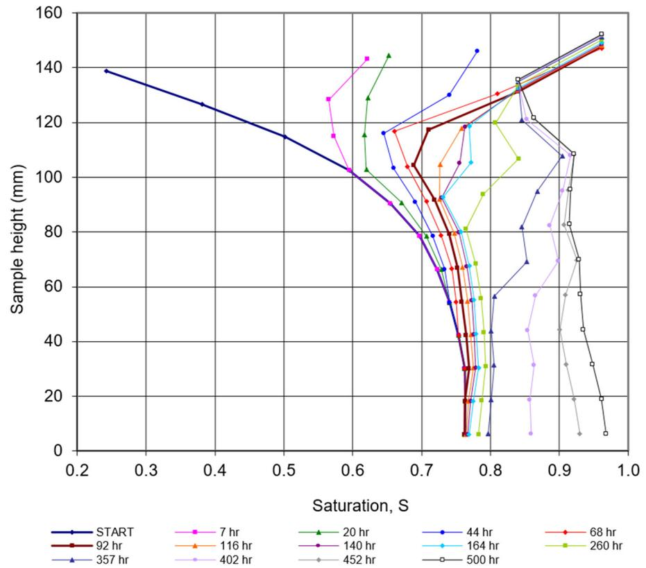
Figure 12. Degree of saturation profiles in the wetting experiment of VU-3.
