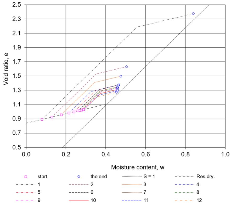
Figure 13. Assumed swelling curves in the wetting experiment of VU-3.
