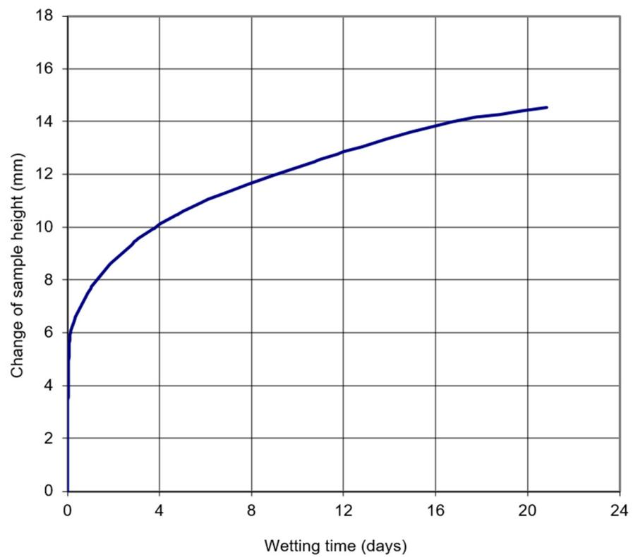
**Figure 9.** Changes in the height of the VU-3 during the wetting experiment.
