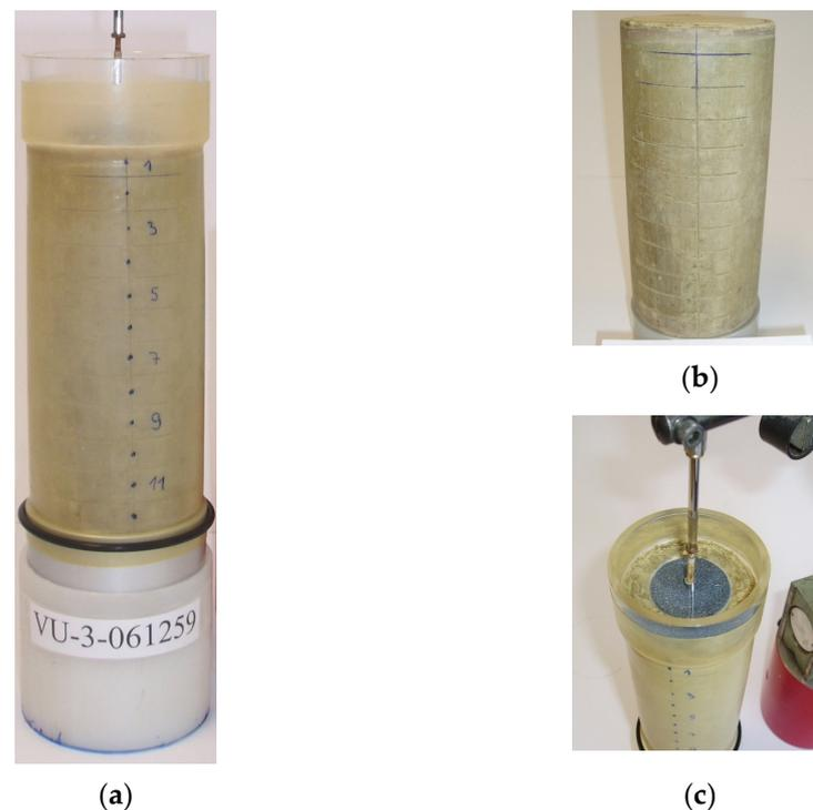
**Figure 6.** Preparation of VU-3 for the 1D wetting phase: (a) the VU-3 on the stand with the cylinder on the top; (b) the VU-3 without the rubber membrane with the engraved marks; (c) the cylinder on the top filled with water at the start of the wetting phase.
