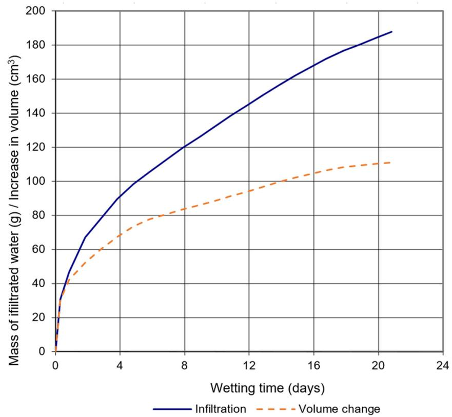
**Figure 8.** Changes in the mass of infiltrated water and changes in the sample volume during the wetting experiment.
