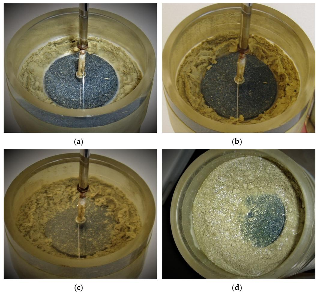
**Figure 14.** Top surface of VU-3 at different times after the start of the wetting phase: (a) 1 min; (b) 3 min; (c) 60 min; (d) 21 days.
