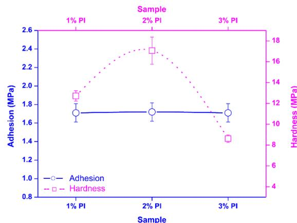
Figure 3. Adhesion and hardness of high refractive index (HRI) coatings with different PI concentrations.
