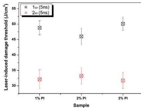
**Figure 4.** 1ω and 2ω laser-induced damage threshold (LIDT) of HRI coatings with different PI concentrations.
