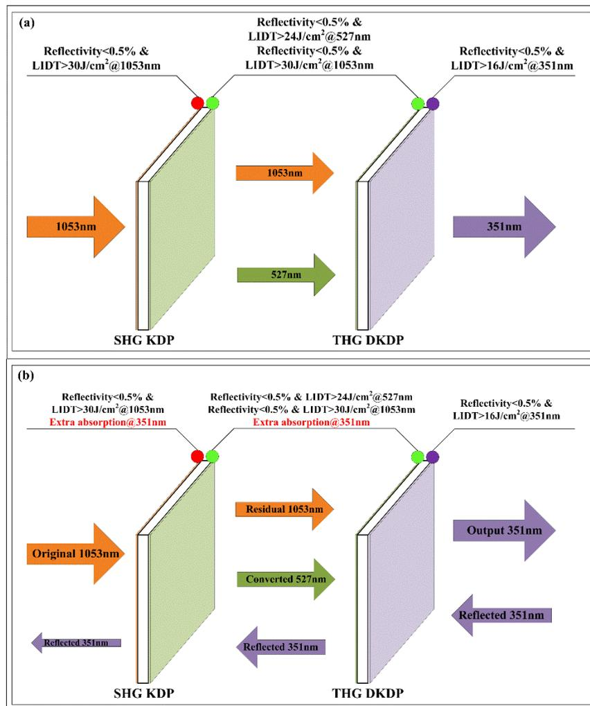
**Figure 1.** Schematic diagram of the frequency-converting pair (FCP) in one laser beam from high-power laser system, (a) original design; (b) optimized design.
