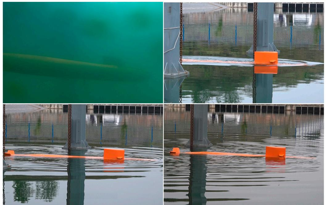
**Figure 8.** The submarine state at different time points during the free ascent experiment.
