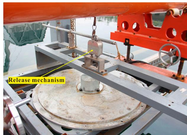
**Figure 5.** Submarine release mechanism.
