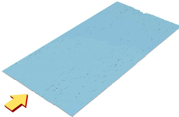
**Figure 4.** The optimized 3D profile of the metasurface waveguide structure. The direction indicate by the yellow arrow is the direction of the incident light.
