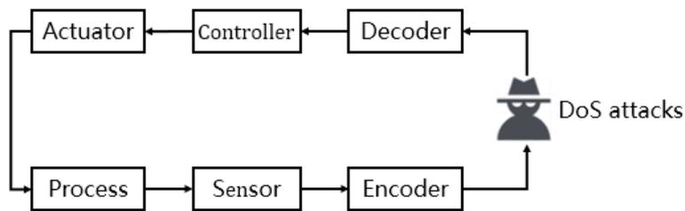
Figure 1. Control architecture of AIOT systems with DoS attacks.
