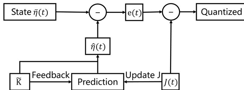
Figure 3. Model-based prediction of the encoder.
