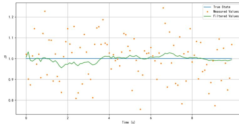
**Figure 7.** The state predicted by the Kalman filter.
