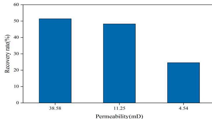
**Figure 10.** Huff-and-puff efficiency for cores with different permeabilities.
