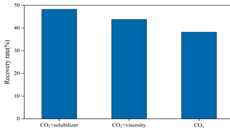
**Figure 6.** Effects on recovery efficiency results of adding different additives.
