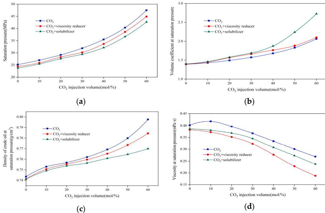
**Figure 4.** (a) The relationship between saturation pressure and amounts of injected CO<sub>2</sub>. Under saturation pressure, the changes in (b) volume coefficient, (c) density, and (d) viscosity of crude oil, with varying amounts of injected CO<sub>2</sub>.
