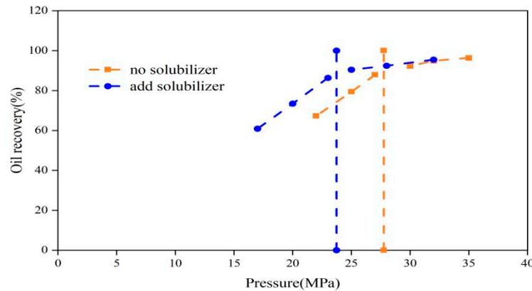
**Figure 5.** Results of experiment on minimum miscibility pressure between crude oil and CO<sub>2</sub>.
