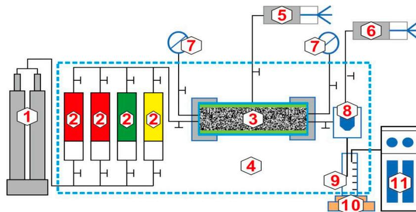
**Figure 3.** Diagram of CO<sub>2</sub> miscible throughput experimental device: (1) ISCO pump; (2) live oil/dead oil/formation water/CO<sub>2</sub>; (3) core holder; (4) constant temperature oven; (5) surrounding-pressure pump; (6) back-pressure pump; (7) pressure sensor; (8) back-pressure valve; (9) gas–liquid separator; (10) electronic balance; (11) gas meter.
