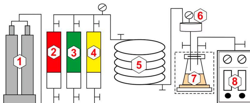
**Figure 2.** Schematic diagram of the minimum miscibility pressure experimental device: (1) ISCO pump; (2) live oil; (3) dead oil; (4) CO<sub>2</sub>; (5) slim tube; (6) back-pressure valve; (7) gas-liquid separator; (8) gas meter.
