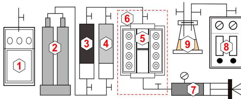
**Figure 1.** Schematic diagram of the PVT experimental device: (1) chromatograph; (2) ISCO pump; (3) oil; (4) CO<sub>2</sub>; (5) PVT visualization tube; (6) temperate box; (7) high-pressure pump; (8) gas meter; (9) gas-liquid separator.
