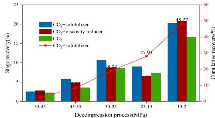
**Figure 7.** Effects on stage recovery of adding different additives in decompression process.
