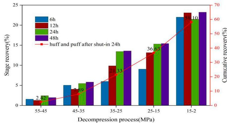
**Figure 9.** Huff-and-puff efficiency results under different discharge pressures.
