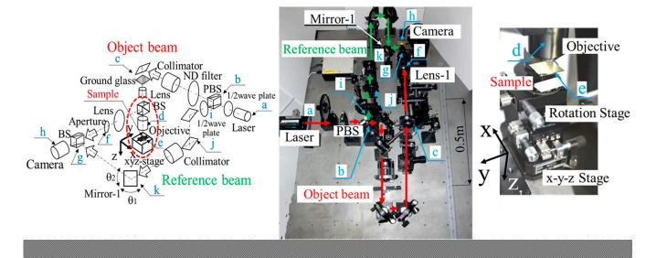
Figure 2. Setup of new optical system. (a) Schematic of optical system. (b) Image of optical system. (c) Sample installation location (within the red dashed line in (a)).
