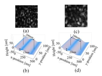
**Figure 6.** Experimental validation of simulation results. (a) Out-of-focus image of a 3600 grids/mm diffraction grating with plane wave illumination. (b) Analysis result of image-(a). (c) Out-of-focus image of a 3600 grids/mm diffraction grating with scattered light. (d) Analysis result of image-(c).
