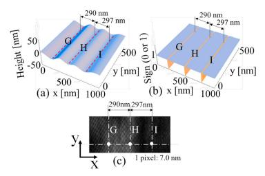
**Figure 14.** Position of the presence of grid of a grating with a period beyond the diffraction limit of the objective lens (3600 grids/mm). (a) Shape of diffraction grating by phase distribution measurement. (b) Minimum position of each groove shape. (c) Estimated position of each groove.
