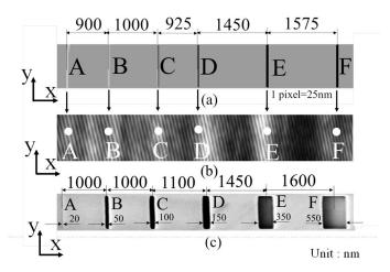
**Figure 13.** Position of the presence of fine lines using the results of Figure 12. (a) Detected position of each groove. (b) Position on speckle pattern. (c) SEM image of each groove.
