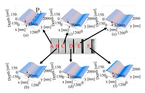
**Figure 12.** Consideration of measurement limits using test sample (scattered light illumination, and F = 1.2 aperture); (a) 20 nm, (b) 50 nm, (c) 100 nm, (d) 150 nm, (e) 350 nm, (f) 550 nm.
