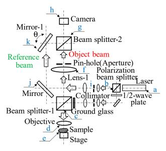
**Figure 1.** Original optical system based on speckle interferometer.
