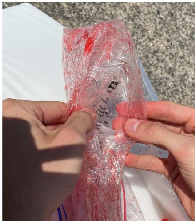
**Figure 12.** IV bag split down long edge (drop test 1).
