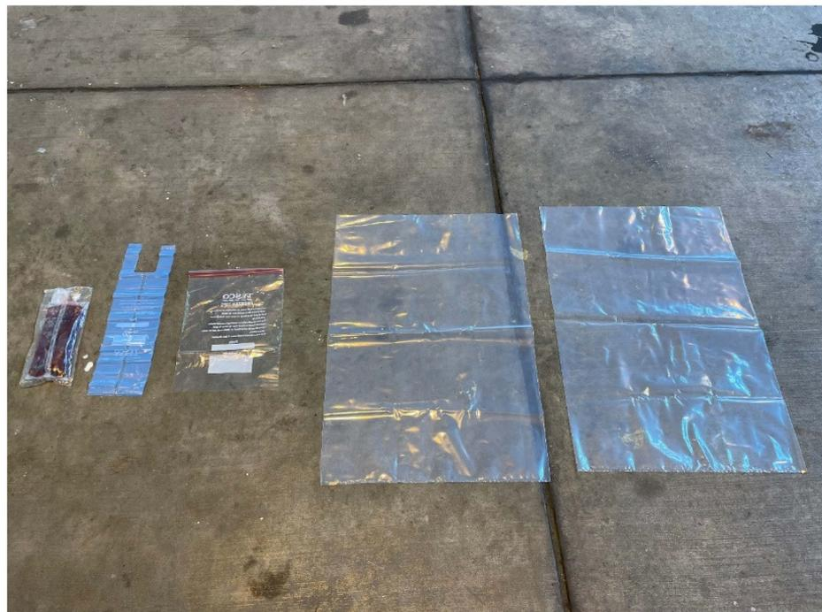
**Figure 6.** Specimen and packaging used in drop tests 3, 6, 7 (IV bag, freezer bag, zip-seal bag, two leak-proof liners) (cold pack not shown).
