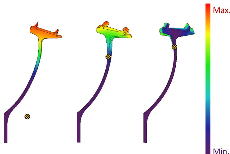
**Figure 10.** Contour plot of the modal displacement module for the 2-fin geometry and torsion centre position. ND 1 (left), ND 3 (centre) and ND 5 (right).
