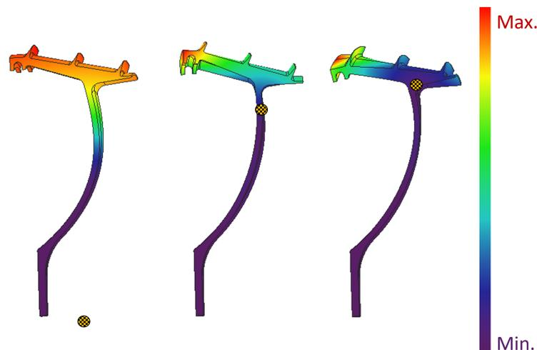
Figure 9. Contour plot of the modal displacement module for the baseline geometry and torsion centre position. ND 1 (left), ND 3 (centre) and ND 5 (right).
