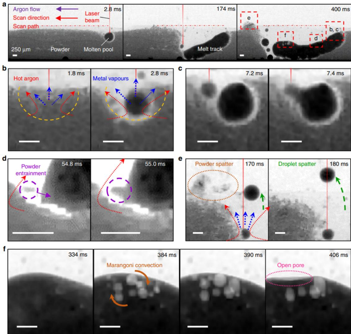
**Figure 8.** Time-series radiographs acquired during LAM of an Invar 36 single-layer melt track (MT1) under  $P = 209\text{ W}$ ,  $v = 13\text{ mm/s}$ , and  $LED = 16.1\text{ J/mm}$  [32].
