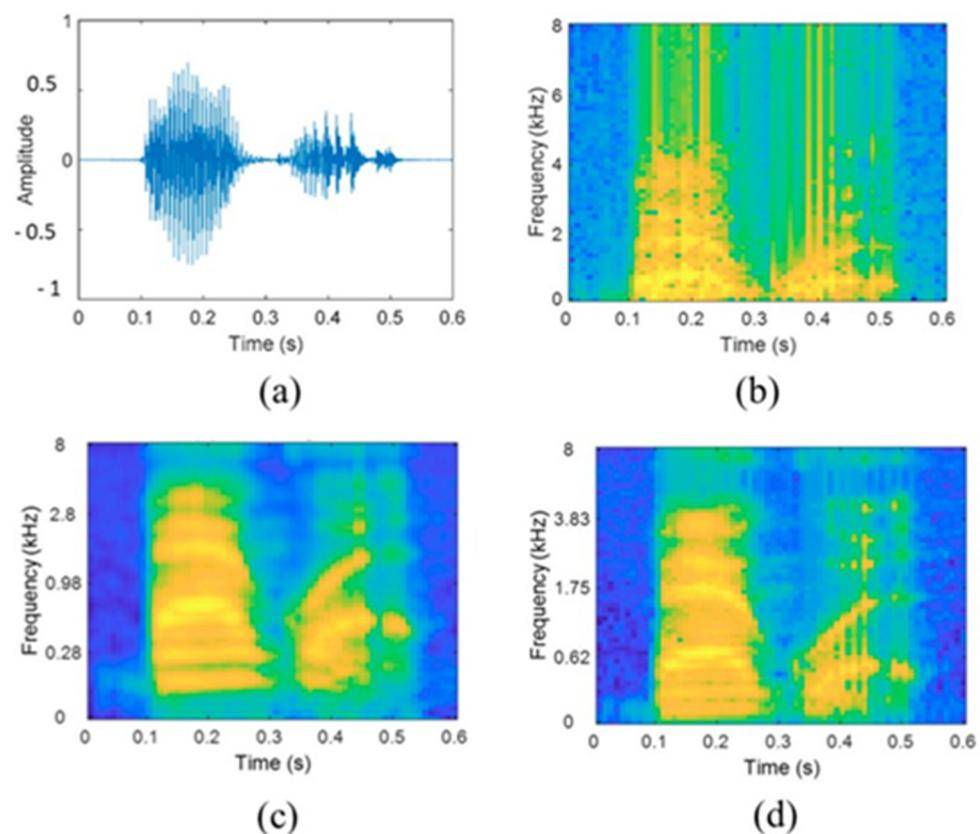
**Figure 12.** Acoustic image representations [36]. (a) acoustic input (b) spectrogram of acoustic input (c) cochleagram of acoustic input (d) Mel spectrogram of acoustic input.
