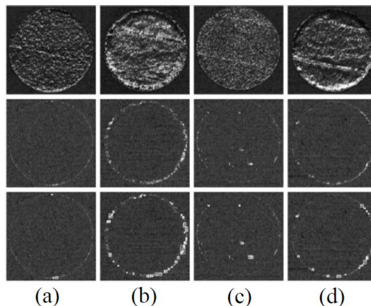
**Figure 5.** From top to bottom: cylinder sample surface image, next powder layer, and detected super-elevations. (a) Reference, (b) laser power +40%, (c) laser power −40%, and (d) hatch distance −40% [30].
