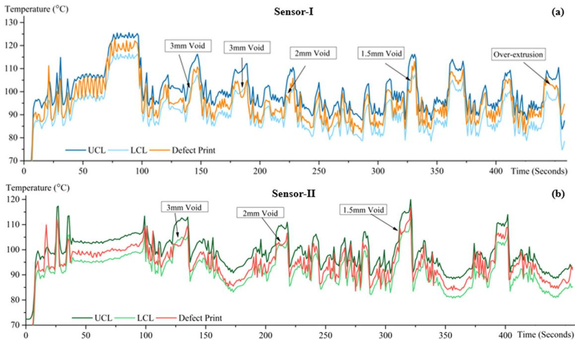
Figure 10.  $\pm 3\sigma$  control chart comparing defected print temperature data with control limits [34]. (a) Sensor-I and (b) Sensor-II.
