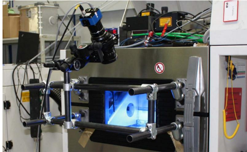
**Figure 4.** The camera setup in front of the LBM machine [30]. The modular tube construction enables flexible positioning with an adjustable height, position, and distance from the door.
