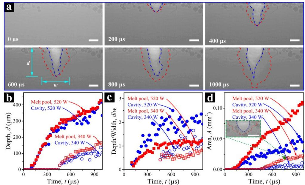
**Figure 3.** Dynamic changes in the melt pool during the laser powder bed fusion process of Ti-6Al-4V [29].
