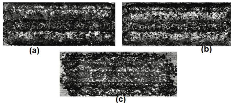
**Figure 13.** Stitched micrograph sample images of each build condition showing differing surface characteristics and surface breaking cracks. (a) Baseline condition, (b) surface roughness influenced by a low-laser-power setting, and (c) significant cracks and rips generated in a low-powder-flow scenario [37].
