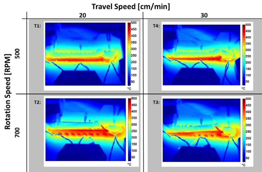
Figure 11. Maps of maximum temperatures assessed for each test [35].
