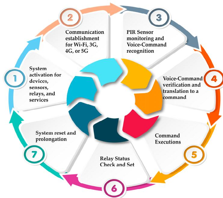
**Figure 3.** A process of seven-step operations designed for the IoT-based smart home and PIR intruder detection system.
