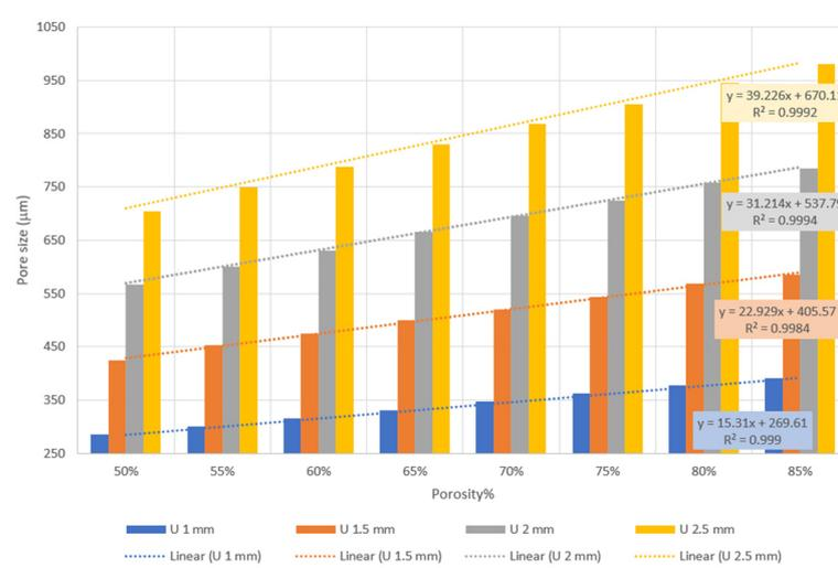
**Figure 1.** Relationship between pore size, unit cell size, and porosity.
