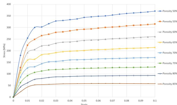
**Figure 2.** Stress–strain curve in the elastic–plastic region of gyroid sheet network with unit cell size 1 mm and porosity between 50 and 85%.
