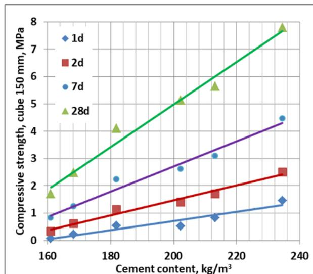
Figure 2. Strength of the applied pumice concrete vs. cement content.
