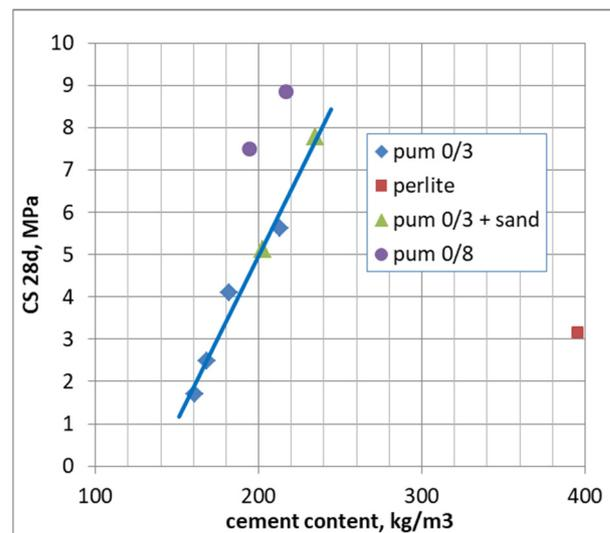
Figure 1. Strength of lightweight concrete vs. the applied pumice concrete vs. cement content.
