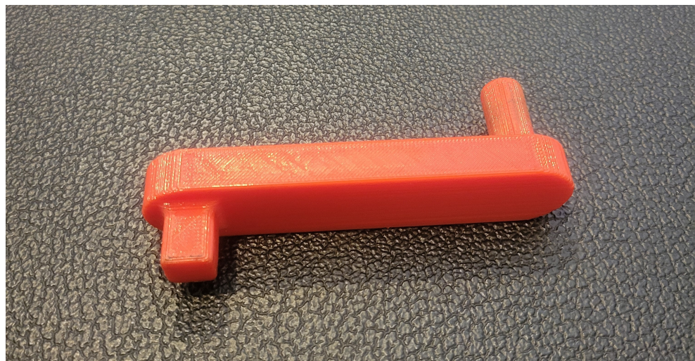
Figure 17. The 3D-printed handle.
