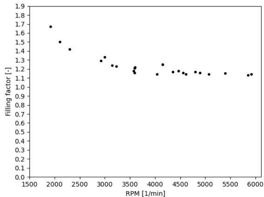
**Figure 8.** Filling factor expressed as a function of the scroll rpm.
