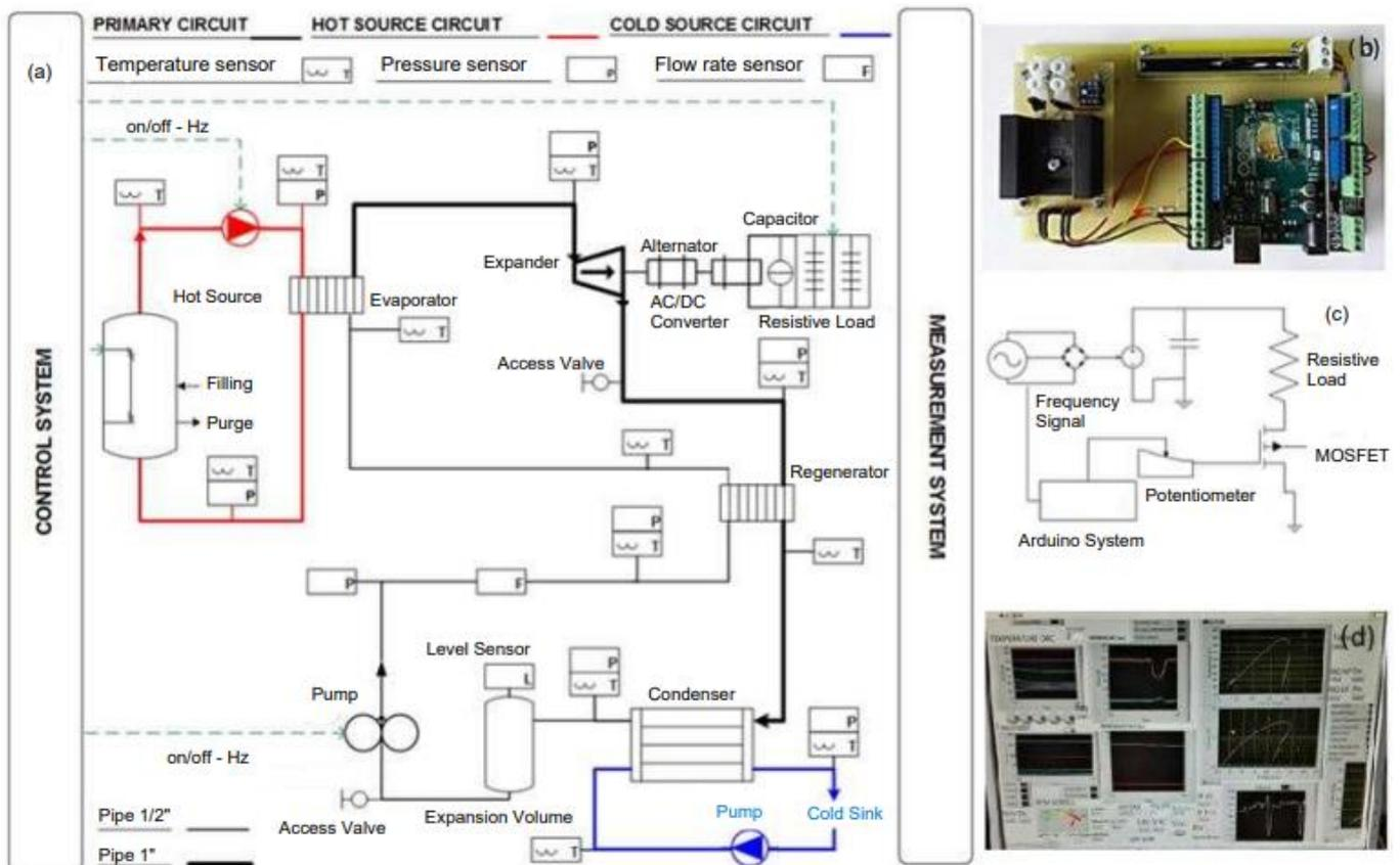
Figure 5. (a) P&I of the test rig, (b) frequency-driven rpm regulator, (c) scheme of the electric control system and (d) user interface of the monitoring software.
