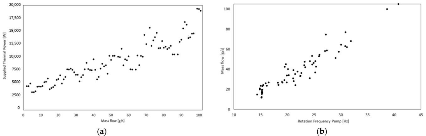
**Figure 7.** (a) Thermal power necessary for the thermodynamic cycle as a function of the working fluid flow rate. (b) Relationship between pump rotation speed and measured flow rate.
