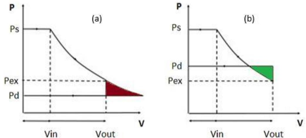
Figure 4. (a) Under-expansion and (b) over-expansion phenomena [26].
