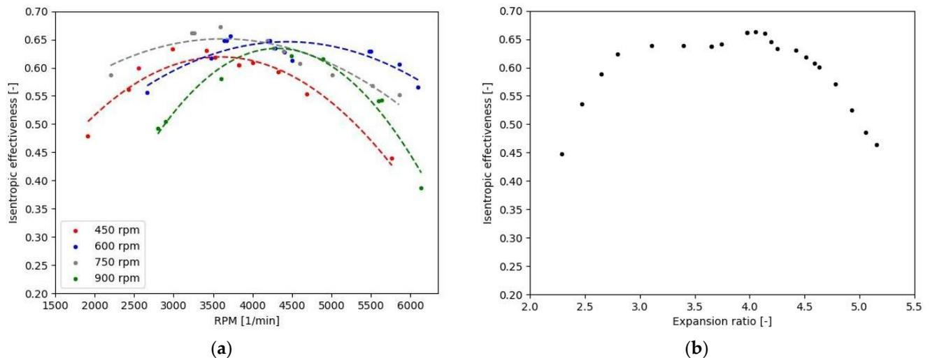
**Figure 6.** Isentropic effectiveness (a) expressed as a function of scroll rpm for different pump speed and (b) expressed as a function of expansion ratio.
