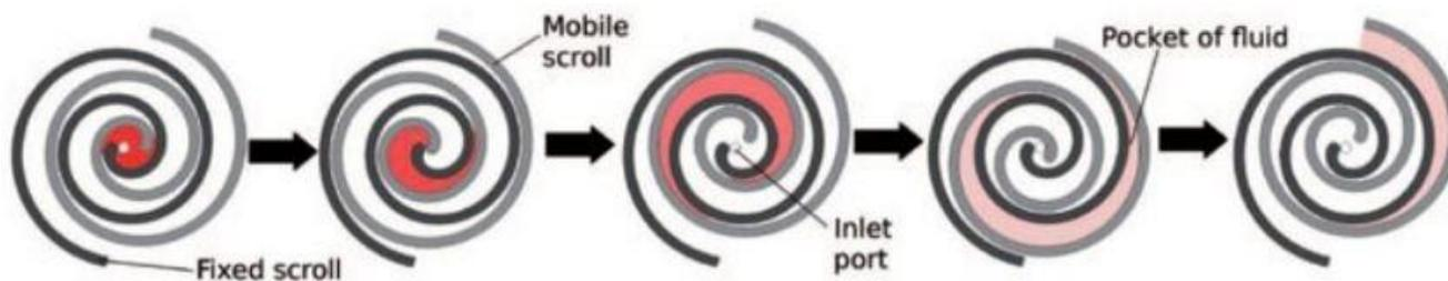
Figure 1. Scroll expander working principle scheme [31].
