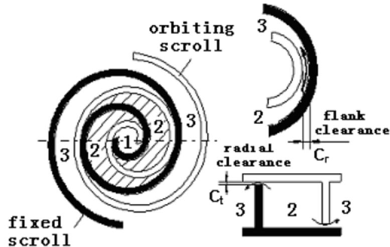
Figure 3. Graphical description of the two different types of leakage causes [39].
