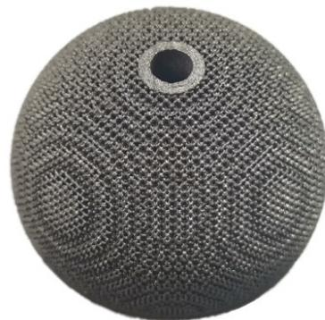
**Figure 15.** Acetabular cup with a gradient porous structure outer surface formed using SLM.
