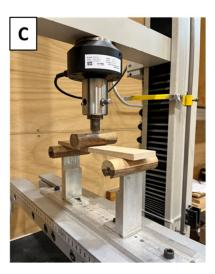
Figure 3. (A) The MTS QTest-5 universal testing machine; (B) IB testing; (C) static bending testing.
