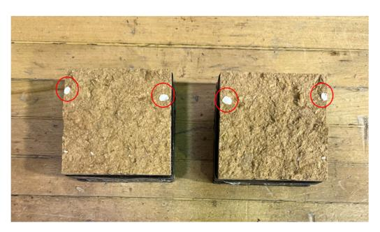
Figure 7. MPCM aggregates formed during panel fabrication.
