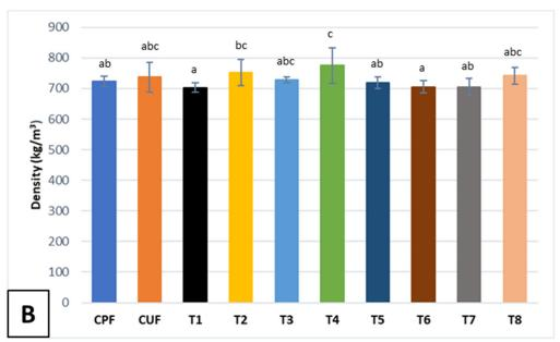
**Figure 4.** Density of the MDF residue-PCM panels. (A) The VDPs of the manufactured panels; (B) the average density of the manufactured panels according to the QDP-01X densitometer. The panel type acronyms are defined in Table 2. The lowercase letters represent statistically significant differences between panel types according to the Tukey test.
