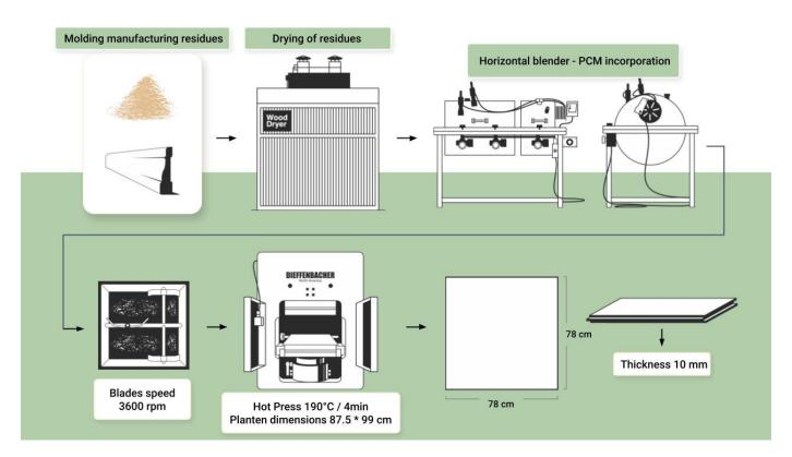
Figure 2. The process used to manufacture the MDF residue-PCM panels.
