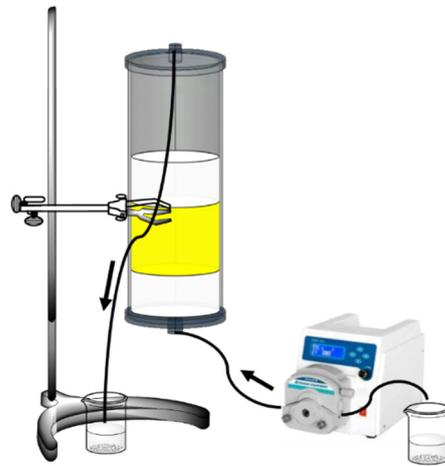
Figure 1. Experimental device diagram.
