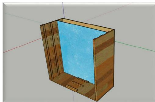
**Figure 5.** Wooden box (dimensions  $750 \times 750 \times 300 \text{ mm}$ ) with a movable PVC partition made for forming biomaterial plates with a thickness of 100, 200, and 300 mm [10].
