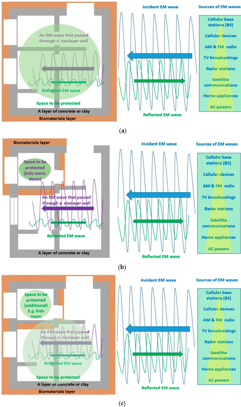
**Figure 3.** Floor plan of a building coated with a biomaterial protective layer: (a) completely coated from the outside; (b) only the room to be protected is coated; (c) the building is completely coated from the outside plus the room to be protected is coated.
