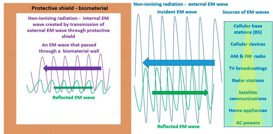
**Figure 2.** EM shielding—a basic method for protection against non-ionizing radiation.
