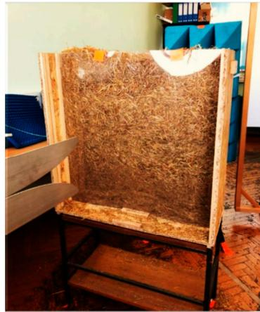
**Figure 6.** Photo of measuring EM wave transmission parameters through biomaterial (wheat harvest residues) in a room with EM reverberation using two Vivaldi antennas: the UWB-2, RFSPACE, Atlanta; GA, USA and RF Analyzer, Fieldfox Handheld N9914A, KEYSIGHT, Santa Rosa, CA, USA [23].
