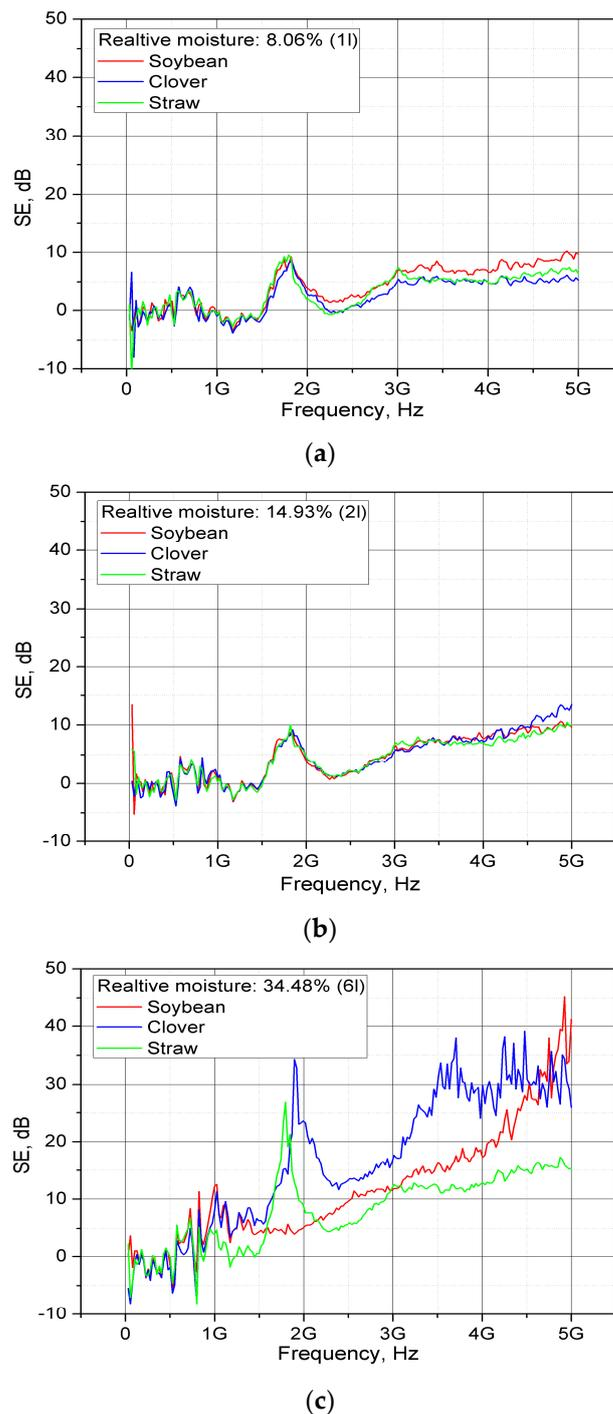
**Figure 10.** Measured SE of soybean straw, wheat straw, and clover straw samples at various levels of relative humidity: (a) 8.06%; (b) 14.93%, and (c) 34.48% (sample thickness 300 mm).
