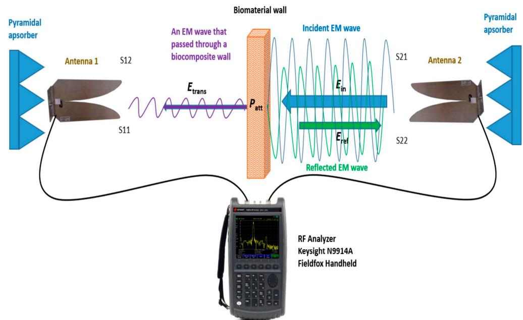
**Figure 1.** Scheme of measurement of EM wave transmission parameters  $S_{21}$  through harvest residues. Antennas 1 and 2 are identical UWB Vivaldi antennas with a gain of 14.7 dBI.
