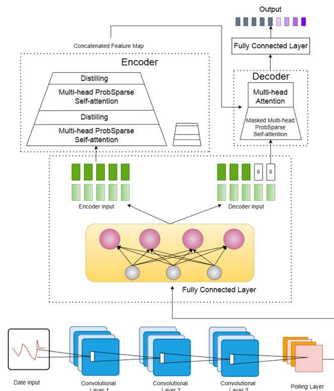
Figure 2. CNN–Informer schematic diagram.
