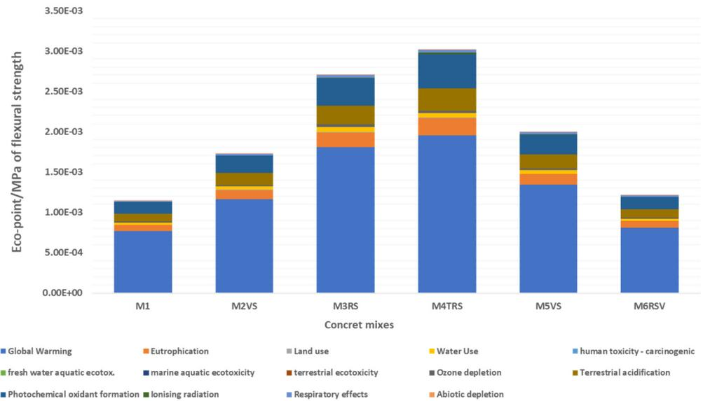
Figure 3. Environmental impacts of six concrete mixes in terms of ‘eco-points’.
