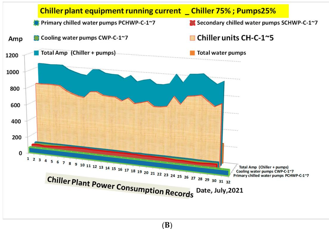
**Figure 11.** (A) The distribution of electrical loadings; (B) the operating current for chiller plant main equipment.
