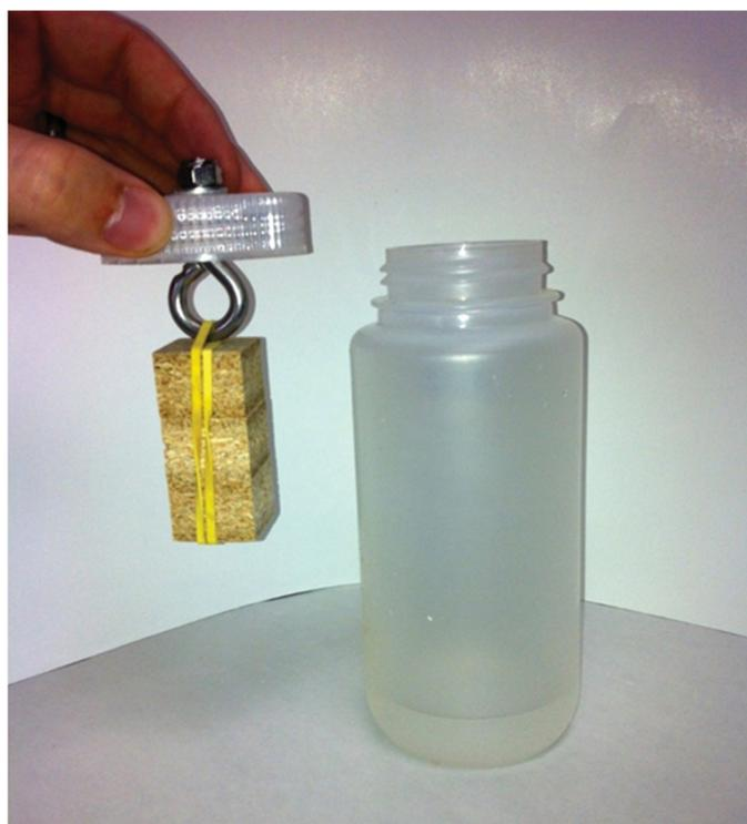
**Figure 3.** Sample setup for modified EN-717-3 method [44].
