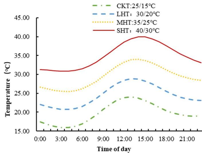
Figure 2. Air temperature dynamics of artificial climate chamber (24 h).
