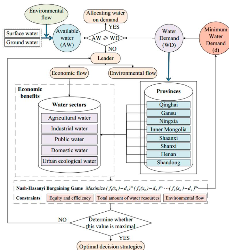
Figure 3. The framework for the design and planning of the Yellow River’s water resources allocation.
