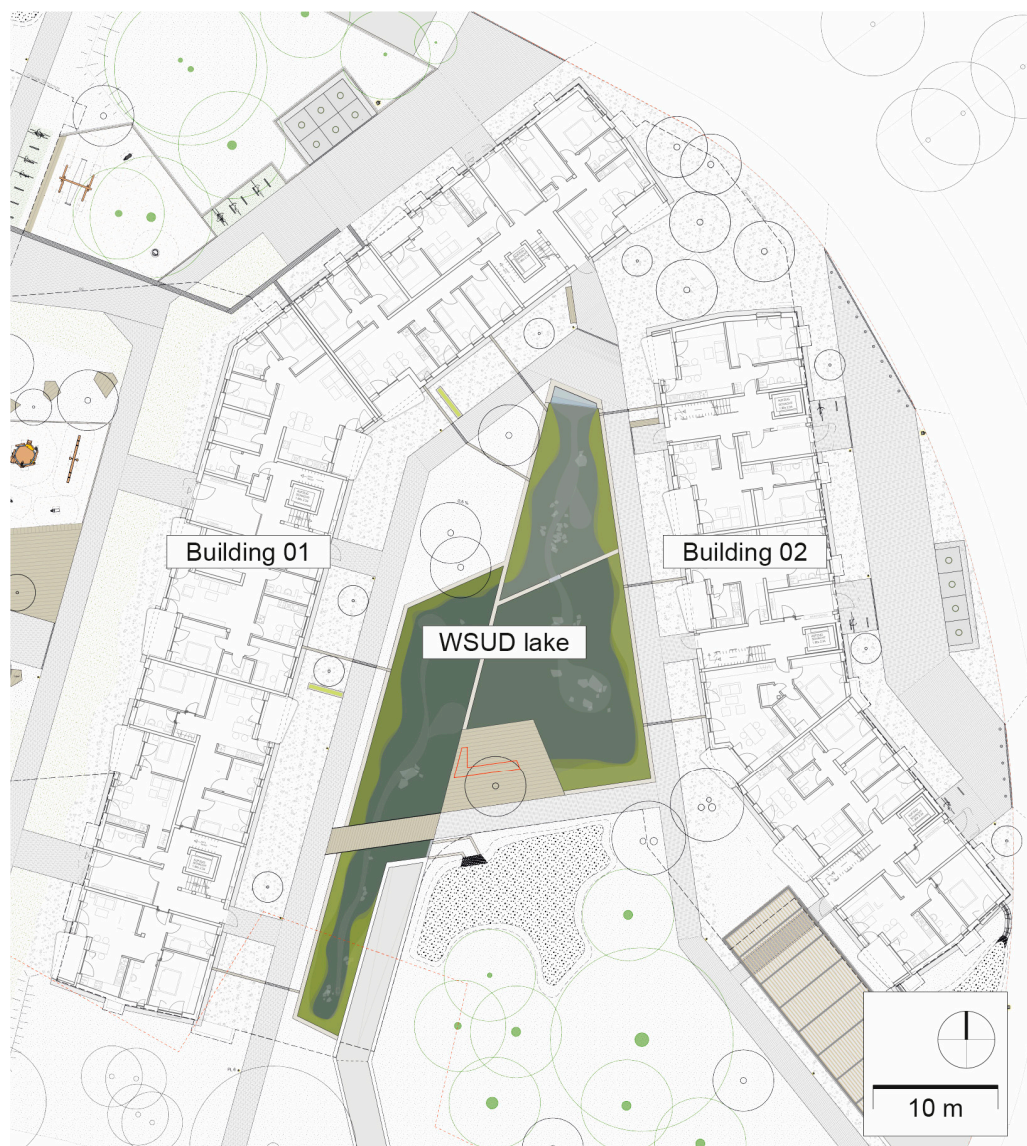
Figure 1. Site plan WSUD prototype.
