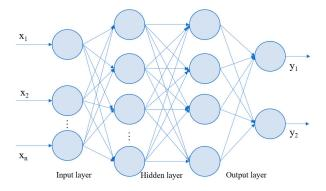
Figure 5. Logic structure diagram of multi-layer perceptron.
