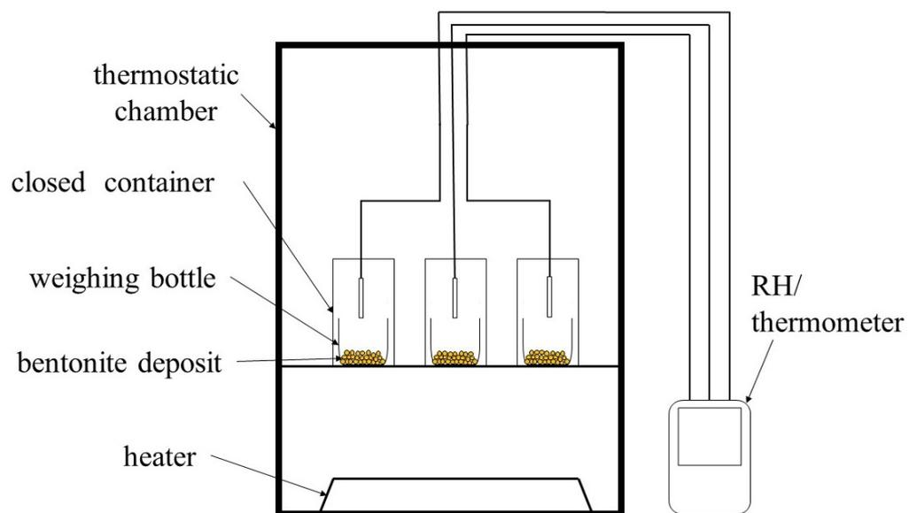
**Figure 8.** Ca-montmorillonite water dehydration experiment.
