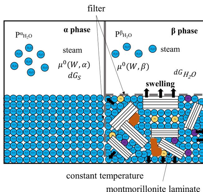
**Figure 5.** A conceptual model of the chemical potential balance of water in the equilibrium state between pure water ( $\alpha$  phase) and water-saturated bentonite ( $\beta$  phase) through a sintered stainless steel filter at a constant temperature.
