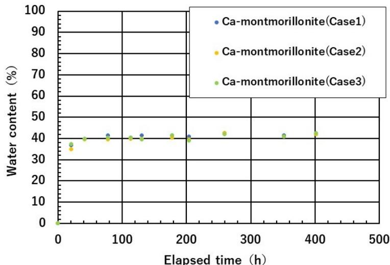
Figure 9. Relationship between elapsed time and water content in water adsorption experiments.
