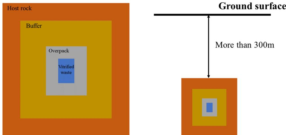
Figure 2. Overview of geological disposal (the left figure shows an overview of engineered barriers and the right figure shows an overview of geological disposal).
