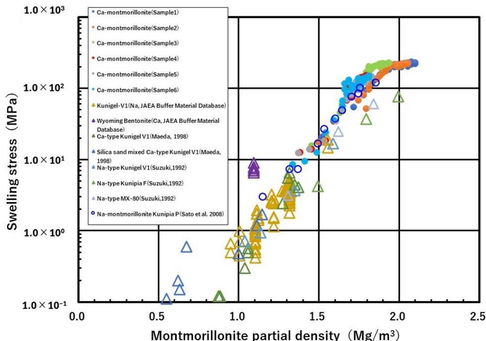
Figure 14. Relationship between montmorillonite partial density and swelling stress [10,18,25,26].
