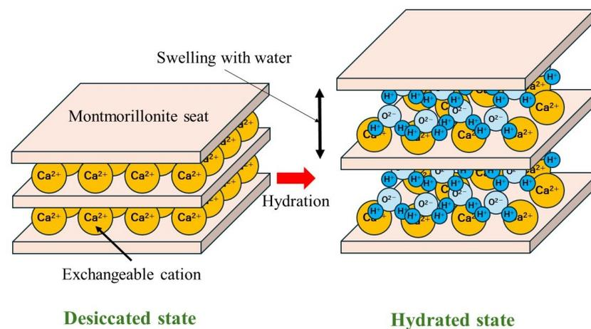
**Figure 4.** Montmorillonite swelling principle.
