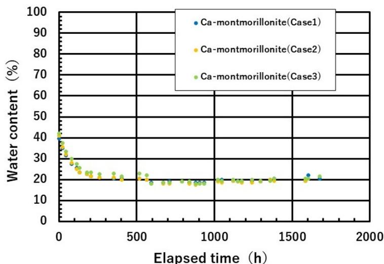
Figure 10. Relationship between elapsed time and water content ratio in water desorption experiments.
