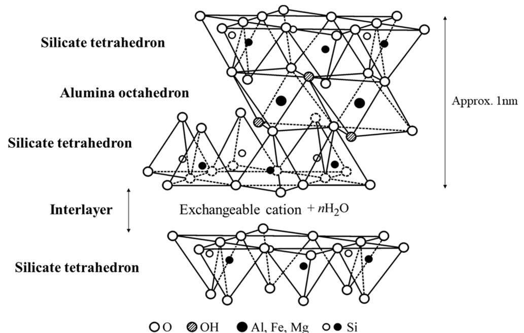
Figure 3. Crystal structure of montmorillonite [4] (partially modified).
