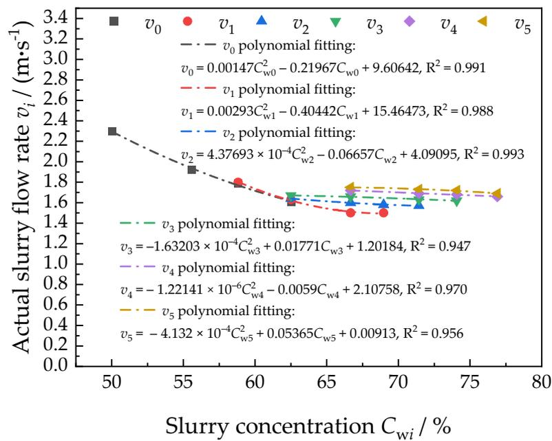
**Figure 5.** Relationship between actual flow rate  $v_i$  and mass concentration  $C_{wi}$  of coal gangue slurry with different gradations.
