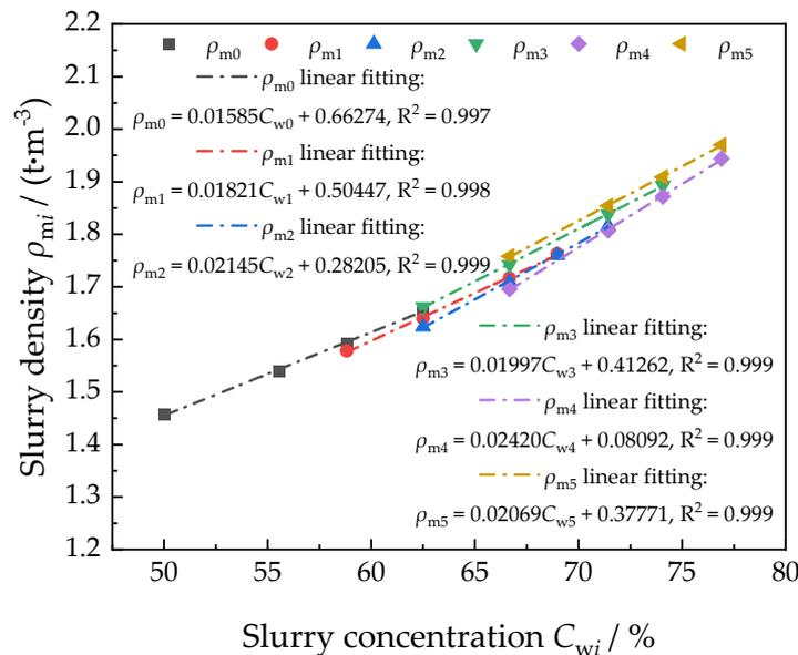
Figure 3. Relationship between density  $\rho_{mi}$  and mass concentration  $C_{wi}$  of coal gangue slurry with different gradations.
