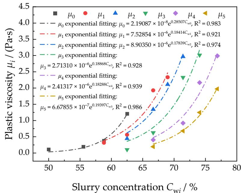
**Figure 6.** Relationship between plastic viscosity  $\mu_i$  and mass concentration  $C_{wi}$  of coal gangue slurry with different gradations.
