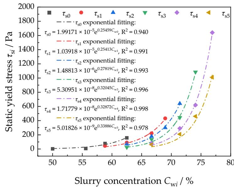
Figure 2. Relationship between static yield stress  $\tau_{si}$  and mass concentration  $C_{wi}$  of coal gangue slurry with different gradations.
