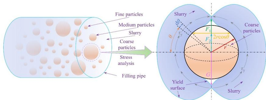
Figure 1. Static force analysis of coarse gangue particles.
