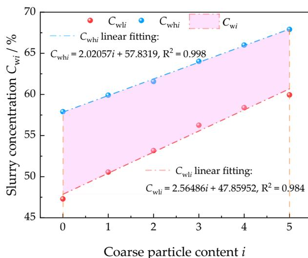
**Figure 7.** Relationship between the minimum transportable concentration  $C_{wli}$ , the maximum transportable concentration  $C_{whi}$ , and the coarse particle content  $i$ .
