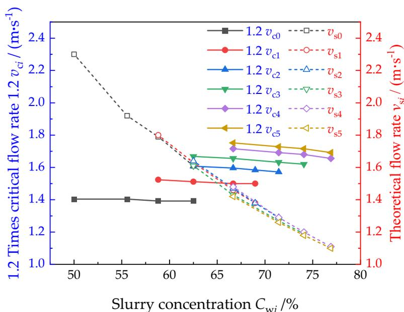
Figure 4. Relationship between 1.2 times the critical flow rate  $1.2 v_{ci}$ , theoretical flow rate  $v_{si}$ , and mass concentration  $C_{wi}$  of coal gangue slurry with different gradations.
