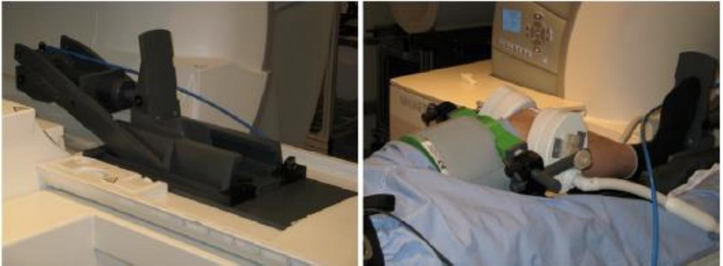
**Figure 2.** Experimental Setup. The knee is loaded with an MR-compatible pneumatic loading device (left). The multipurpose coil is attached to the thigh and the tracking marker for prospective motion correction is taped to the knee cap (right).
