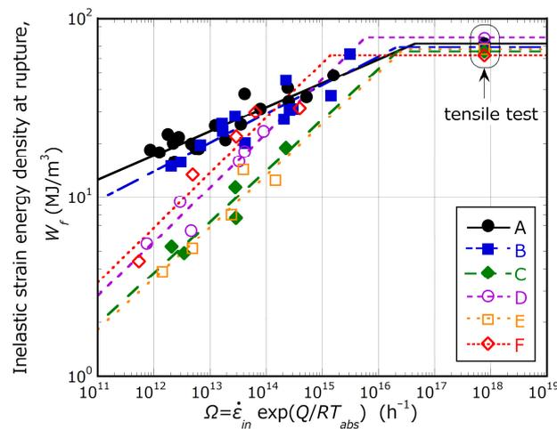
**Figure 15.** Relationship between inelastic strain energy density at rupture and strain rate–temperature parameter. Each line was used in calculation of creep damage for the hybrid approach. The value of activation energy was set as  $2.98 \times 10^5$  J/mol using the NIMS creep database including various heat and temperature data.
