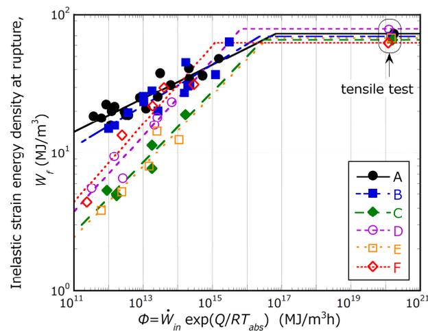
**Figure 14.** Relationship between inelastic strain energy density at rupture and inelastic strain energy density rate–temperature parameter. Each line was used in calculation of creep damage for the energy-based approach. The value of activation energy was set as  $2.60 \times 10^5$  J/mol using the NIMS creep database [34] including various heat and temperature data.
