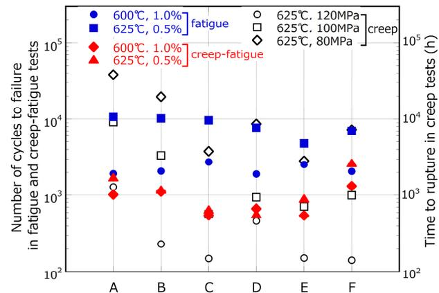
**Figure 11.** Variations in creep, fatigue, and creep-fatigue lives.
