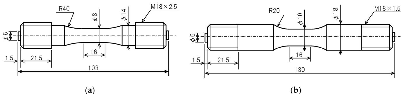
**Figure 2.** Test specimens used for fatigue and creep-fatigue tests (unit: mm). (a) Specimen with 8 mm diameter used in the tests at 625 °C; (b) specimen with 10 mm diameter used in the tests at 600 °C.
