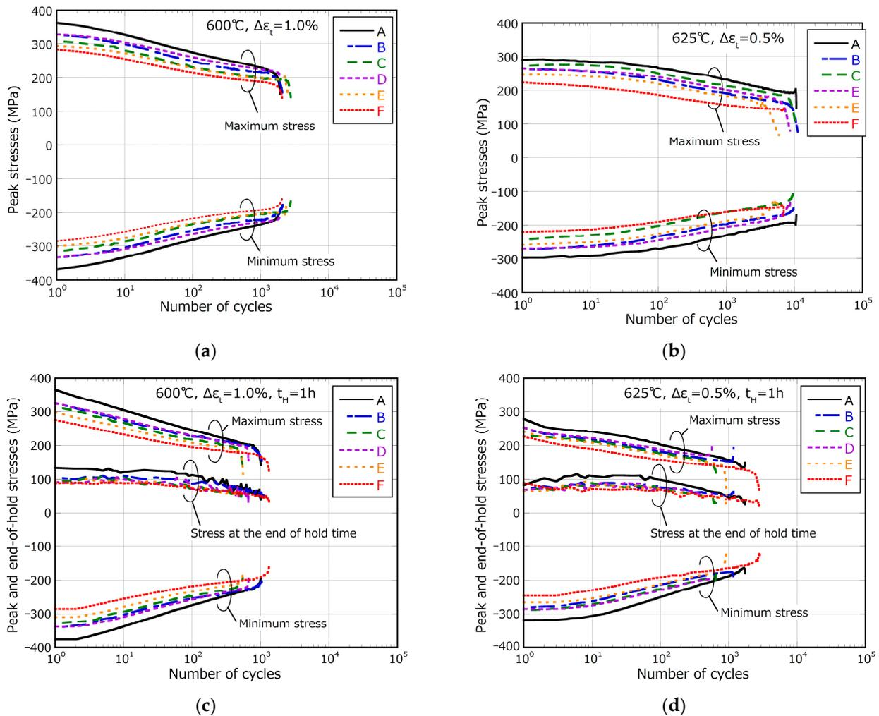
**Figure 8.** Comparison of change in peak stresses in fatigue and creep-fatigue tests in the six materials. The stress at the end of hold time is also displayed for creep-fatigue tests. (a) Fatigue test, 600 °C,  $\Delta\epsilon_t = 1.0\%$ ; (b) fatigue test, 625 °C,  $\Delta\epsilon_t = 0.5\%$ ; (c) creep-fatigue test, 600 °C,  $\Delta\epsilon_t = 1.0\%$ ,  $t_H = 1$  h; (d) creep-fatigue test, 625 °C,  $\Delta\epsilon_t = 0.5\%$ ,  $t_H = 1$  h.
