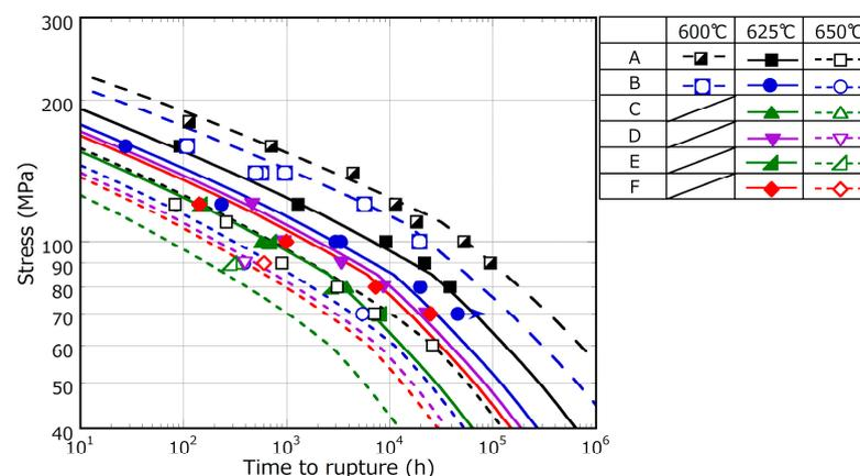
**Figure 12.** Creep test data at various temperatures and regression curves given by Equation (6) and constants in Table 4. Each creep rupture curve was used in calculation of creep damage for the time fraction approach. Note that the constant  $p_0$  of materials C and E is the same value, so their creep rupture curves are the same.
