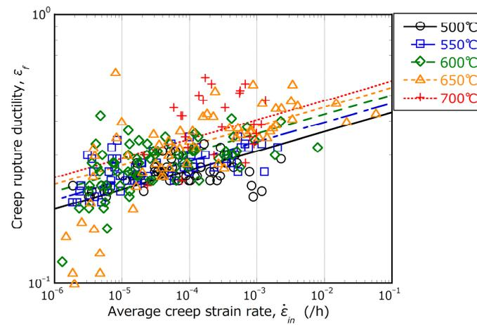
**Figure A1.** Relationship between creep rupture ductility and creep strain rate at representative temperatures in the NIMS creep database. Each line represents a regression line given by Equation (A1) and constants given in Table A1.
