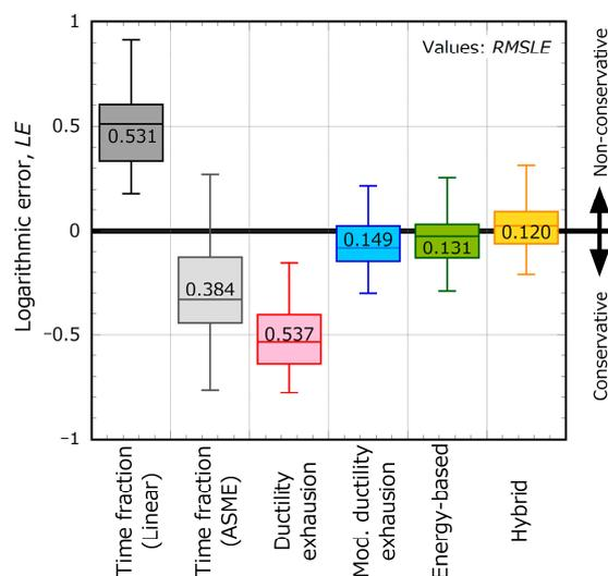
**Figure 18.** Boxplot of logarithmic error for creep-fatigue life evaluation in each approach. Value in each box shows root mean squared logarithmic error calculated by Equation (24).
