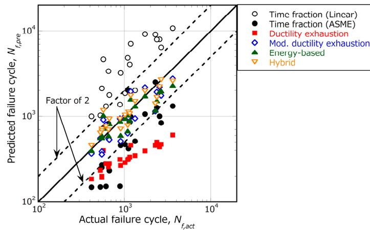
**Figure 17.** Comparison of performance of five approaches in creep-fatigue life estimation. In the time fraction approach, life evaluation results are shown for the cases using the simple linear damage summation rule ( $D_f + D_c = 1$ ) and the ASME creep-fatigue damage envelope.
