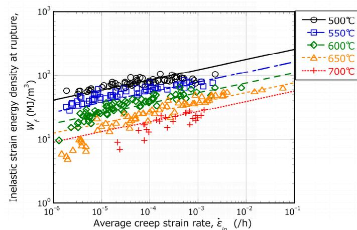
**Figure A3.** Relationship between inelastic strain energy density at rupture and creep strain rate at representative temperatures in the NIMS creep database. Each line represents a regression line given by Equation (A3) and constants given in Table A1.
