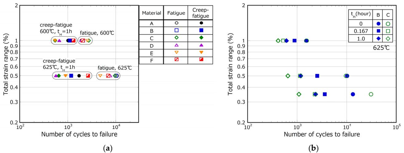
**Figure 6.** Relationship between total strain range and number of cycles to failure for strain-controlled fatigue and creep-fatigue tests. (a) Comparison of failure lives of the six materials; (b) comparison of failure life of materials B and C in various strain-range and hold-time conditions.
