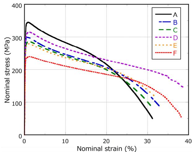
**Figure 3.** Comparison of nominal stress–nominal strain curves of six heats at 625 °C.
