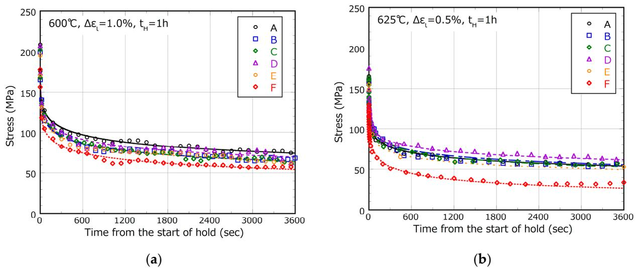
**Figure 10.** Comparison of stress-relaxation behavior at half-life cycles in creep-fatigue tests. (a) 600 °C,  $\Delta\epsilon_t = 1.0\%$ ,  $t_H = 1\text{ h}$ ; (b) 625 °C,  $\Delta\epsilon_t = 0.5\%$ ,  $t_H = 1\text{ h}$ . Each line represents the regression curve given by Equation (3) used for calculating creep damage in creep-fatigue life evaluation.
