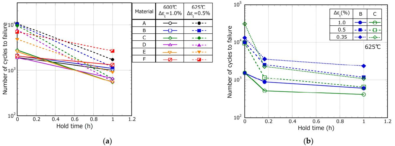
**Figure 7.** Relationship between number of cycles to failure and hold time. (a) Comparison between the six materials under two different conditions; (b) comparison between materials B and C under various strain-range and hold-time conditions.
