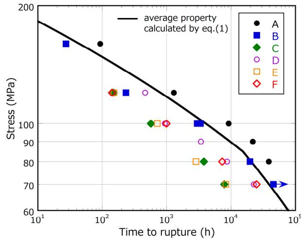
**Figure 4.** Relationship between stress and time to creep rupture at 625 °C. The line represents the average creep rupture property of Grade 91 steel calculated from Equation (1). One test (material B, 70 MPa) is ongoing.
