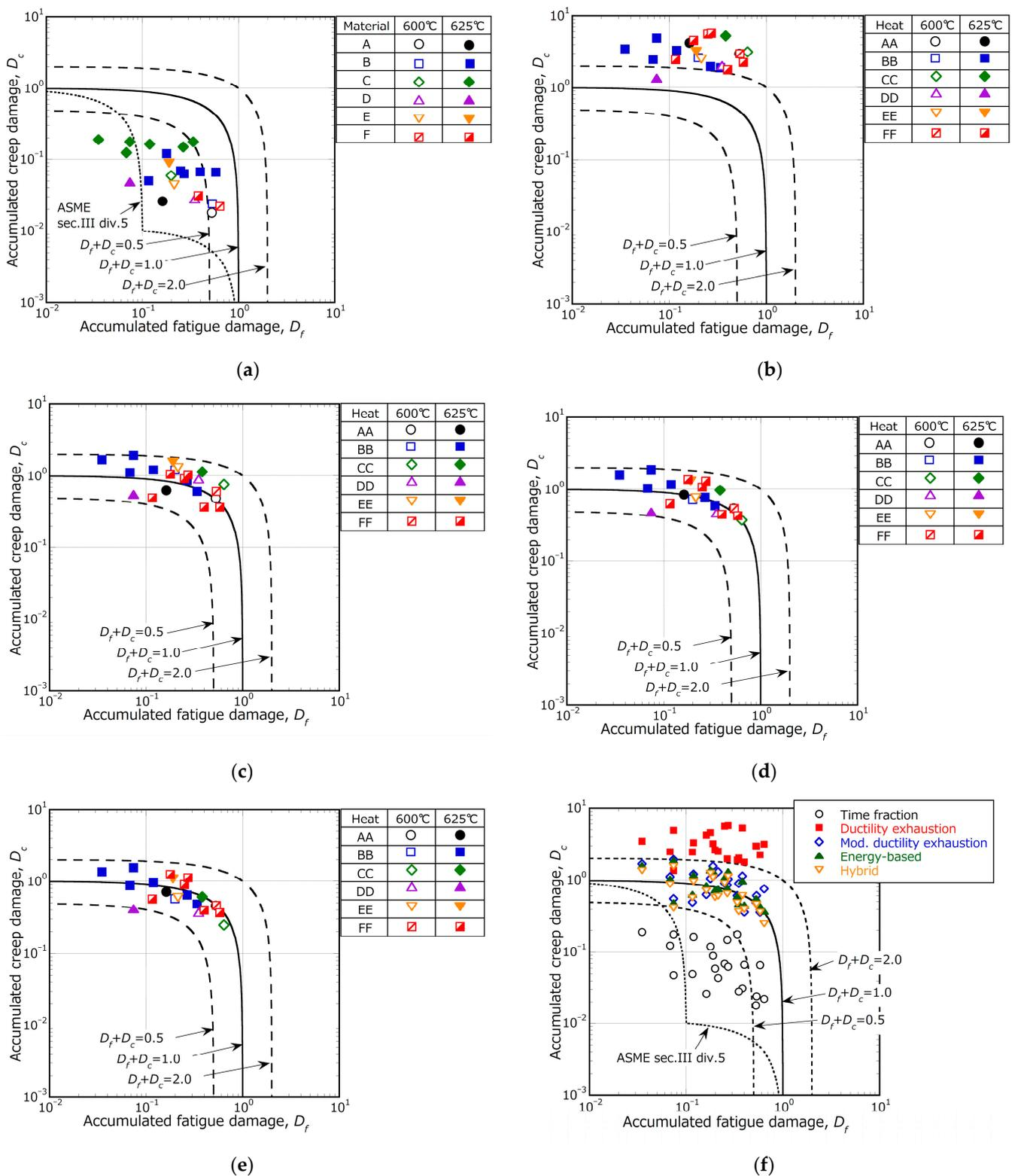
**Figure 16.** Accumulated creep-fatigue damage diagrams in each approach. (a) Time fraction approach; (b) Ductility exhaustion approach; (c) Modified ductility exhaustion approach; (d) Energy-based approach; (e) Hybrid approach; (f) Comparison between the five approaches. The line through  $(D_f = 0.1, D_c = 0.01)$  in (a,f) is used in the ASME BPVC Section III Division 5 as the creep-fatigue damage envelope for Grade 91 steel in the time fraction approach.
