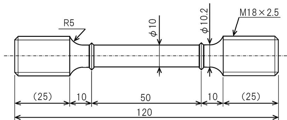
Figure 1. Test specimen used for tensile and creep tests (unit: mm).
