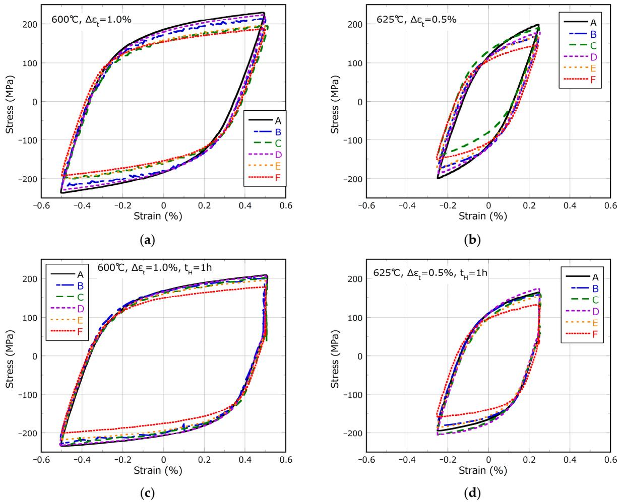
**Figure 9.** Comparison of hysteresis loops at half-life cycles in fatigue and creep-fatigue tests. (a) Fatigue test, 600 °C,  $\Delta\epsilon_t = 1.0\%$ ; (b) fatigue test, 625 °C,  $\Delta\epsilon_t = 0.5\%$ ; (c) creep-fatigue test, 600 °C,  $\Delta\epsilon_t = 1.0\%$ ,  $t_H = 1\text{ h}$ ; (d) creep-fatigue test, 625 °C,  $\Delta\epsilon_t = 0.5\%$ ,  $t_H = 1\text{ h}$ .
