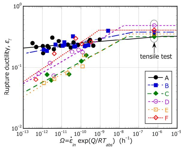
**Figure 13.** Relationship between rupture ductility and inelastic strain rate–temperature parameter. Each line was employed in the calculation of creep damage for both the ductility exhaustion and modified ductility exhaustion approaches. The value of the activation energy was set to  $-1.16 \times 10^5$  J/mol based on the NIMS creep database, which includes various heat and temperature data.
