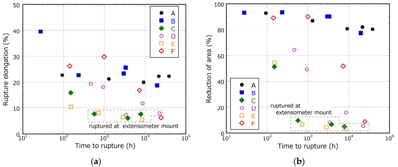
**Figure 5.** Variation of creep rupture ductility with respect to creep rupture time at 625 °C. (a) Rupture elongation; (b) reduction in area. Eight data points with particularly small ductility in materials C, D, and E fractured adjacent to the extensometer mount.
