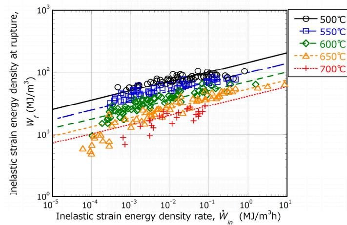
**Figure A2.** Relationship between inelastic strain energy density at rupture and inelastic strain energy density rate at representative temperatures in the NIMS creep database. Each line represents a regression line given by Equation (A2) and constants given in Table A1.
